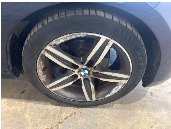
1: Wheel osf Corroded Light
