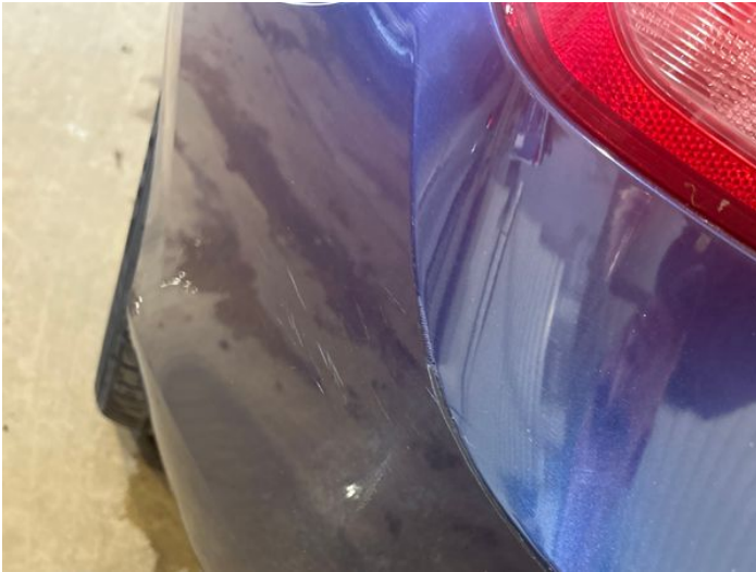
9: Bumper Rear Scratched Over 100mm Thru Paint
