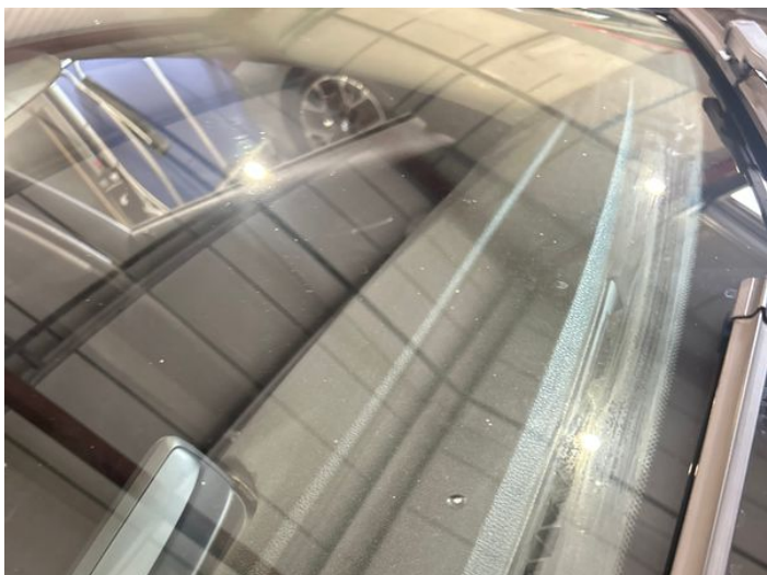
21: Screen Front Chipped UpTo 10mm
