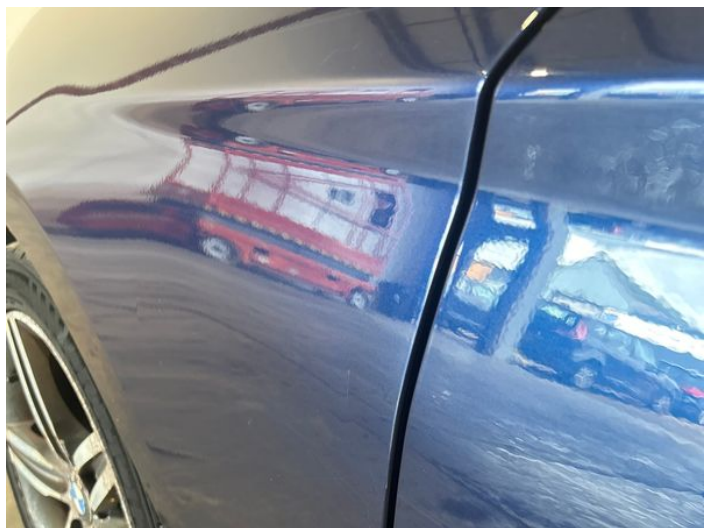
14: Wing nsf Dented Between 10mm + 30mm
