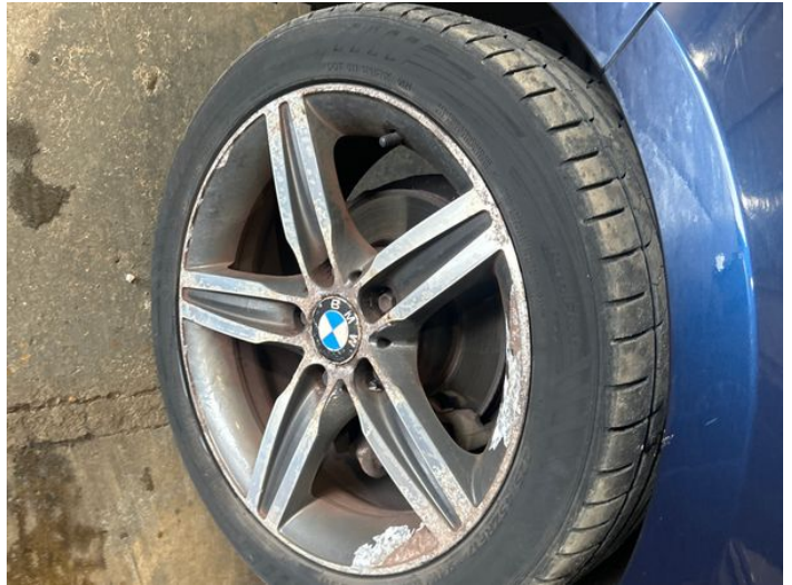
16: Wheel nsf Corroded Light
