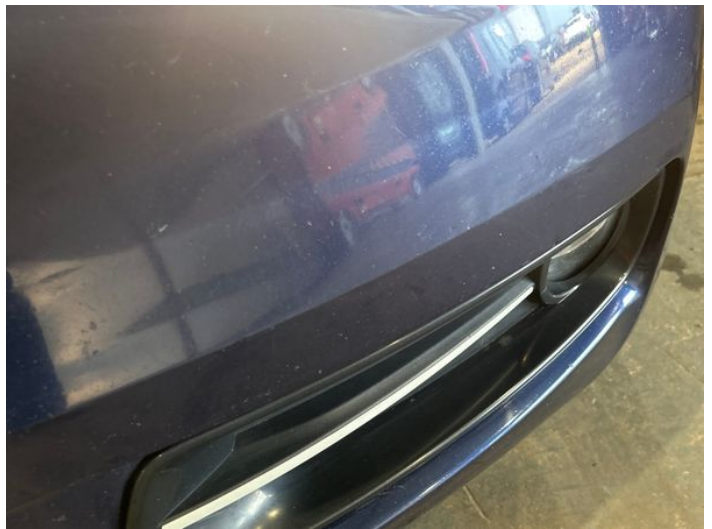
18: Bumper Front Chipped Multiple Chips
