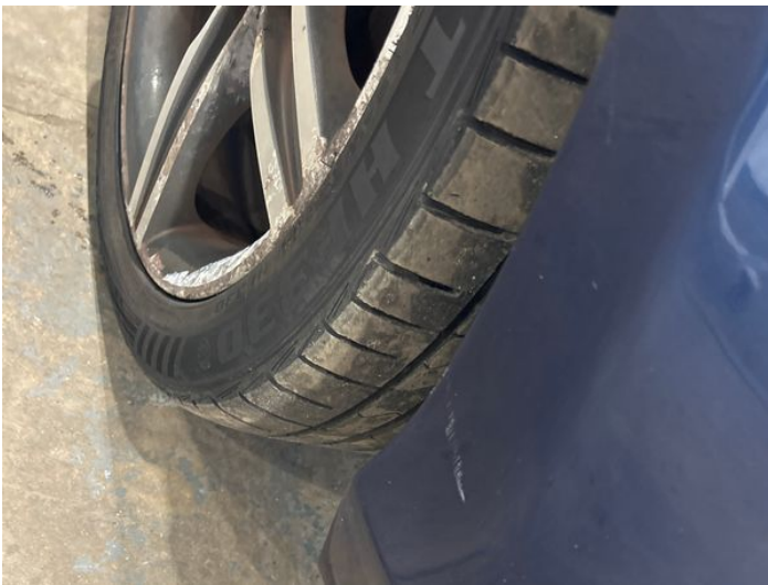
17: Bumper Front Scratched UpTo 25mm Thru Paint
