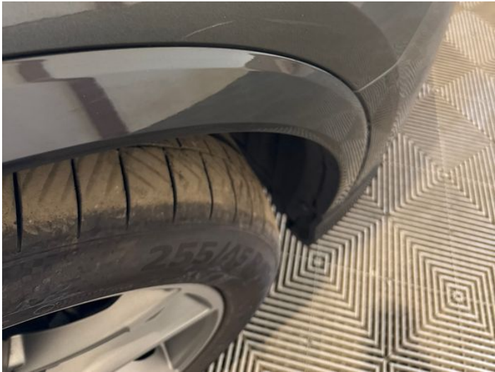
10: Wing osf Scratched Over 25mm Thru Paint
