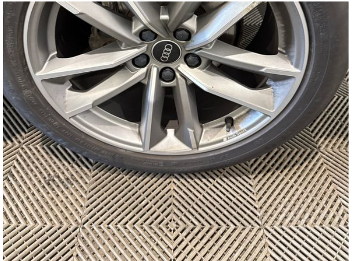
6: Wheel nsr Corroded Light
