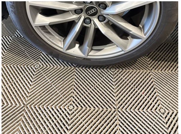
4: Wheel nsf Scratched Up To 50mm
