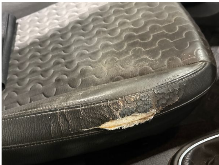
1: Seat Base Cover nsf Torn Over 3mm
