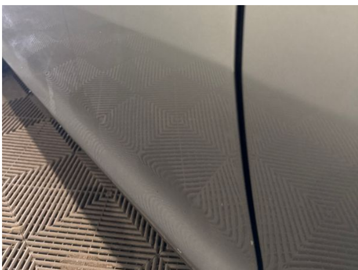
11: Door nsf Scratched UpTo 25mm Thru Paint
