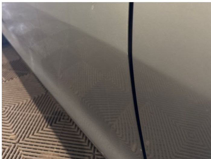
10: Door nsf Dented Between 10mm + 30mm
