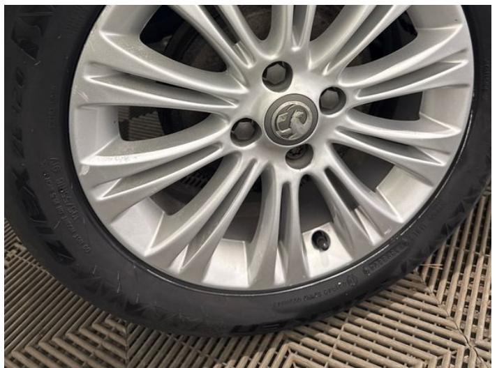
20: Wheel osr Scratched Over 50mm
