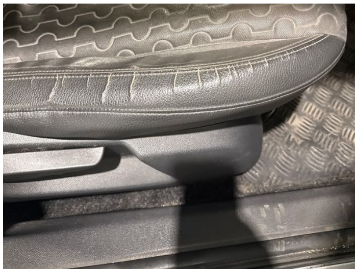
2: Seat Back Cover osf Scuffed Over 25mm
