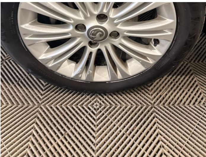
7: Wheel nsf Scratched Over 50mm
