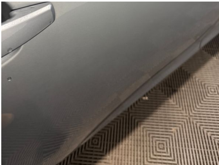
21: Door osr Scratched Over 25mm Thru Paint
