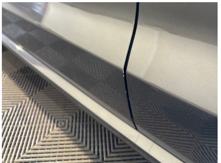
8: Door nsf Chipped Edge Chip
