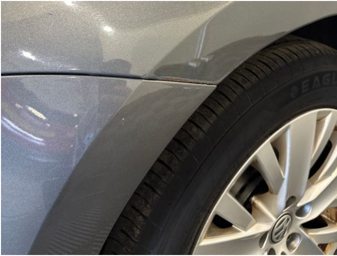
3: Wing nsf Rusted Over 5mm
