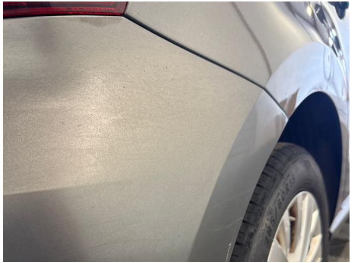
12: Bumper Rear Poor Previous Repair Poor Paint
