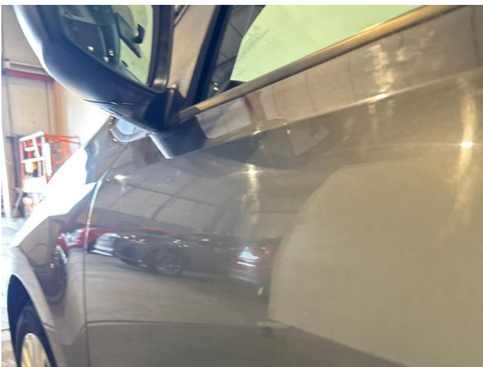
7: Door nsf Dented Over 30mm
