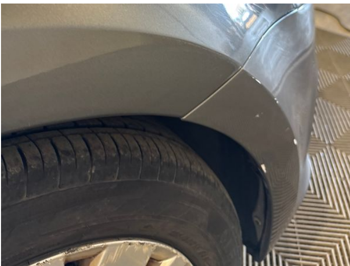
19: Wing osf Scratched Over 25mm Thru Paint
