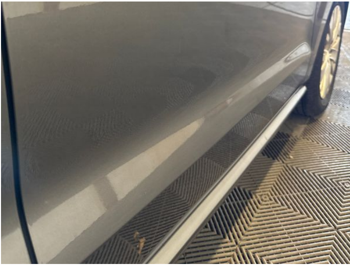
17: Door osf Poor Previous Repair Poor Paint
