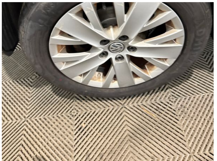
14: Wheel osr Scratched Over 50mm
