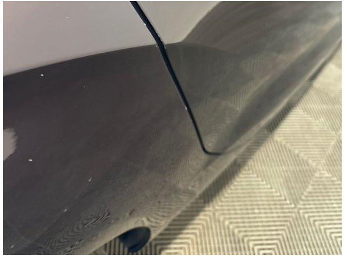
16: Door osr Chipped Edge Chip
