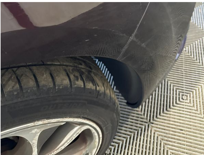
19: Wing osf Scratched Over 25mm Thru Paint
