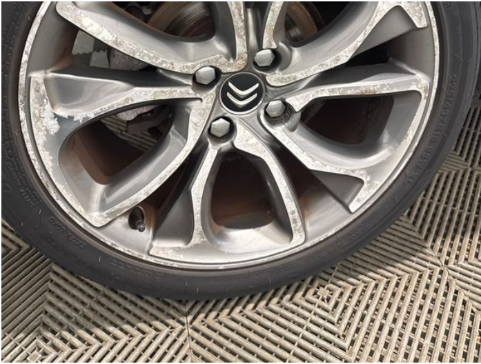
15: Wheel osr Scratched Over 50mm
