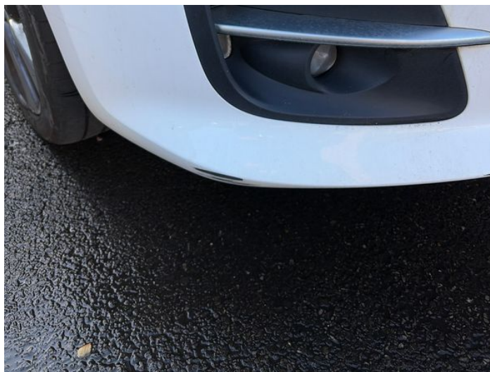
2: Bumper Front Scratched Over 100mm Thru Paint
