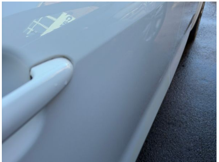
12: Door osr Dented Between 10mm + 30mm
