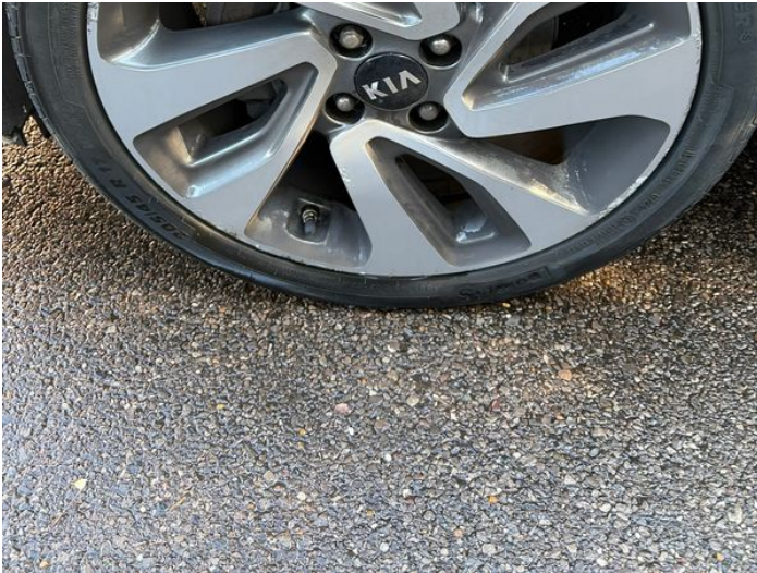
3: Wheel nsf Scratched Over 50mm
