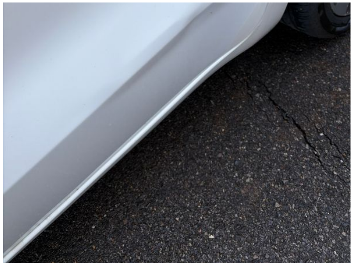
6: Door nsr Dented Over 30mm
