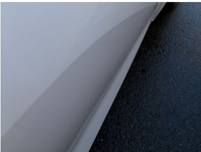
13: Door osf Dented Between 10mm + 30mm
