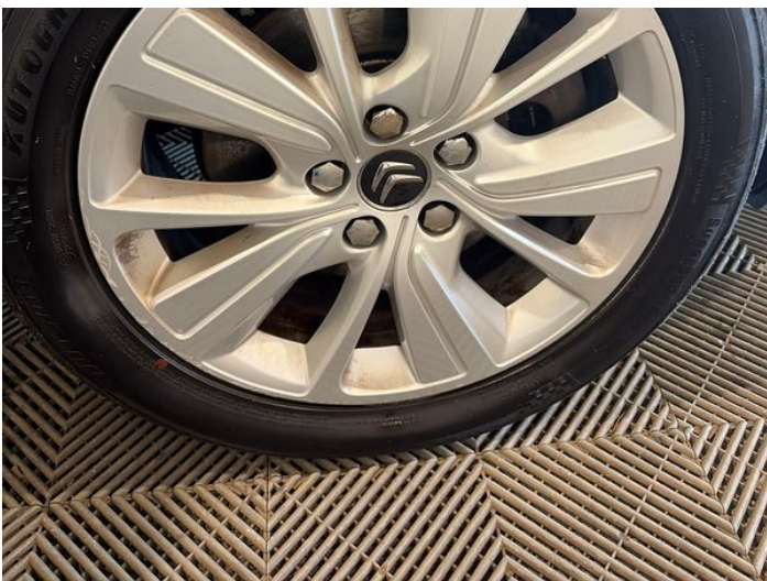
19: Wheel osf Scratched Over 50mm
