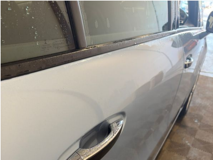
15: Door osr Poor Previous Repair Rippled UpTo 30%
