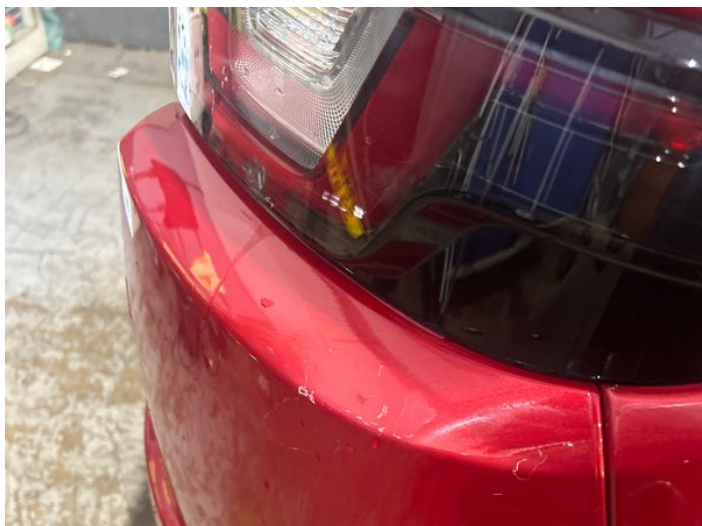
3: Bumper Rear Poor Previous Repair Paint Flake
