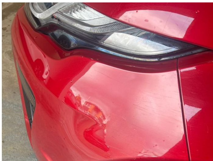
6: Bumper Front Poor Previous Repair Paint Flake
