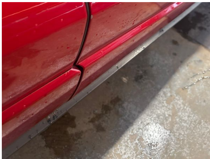
2: Door osf Chipped Edge Chip
