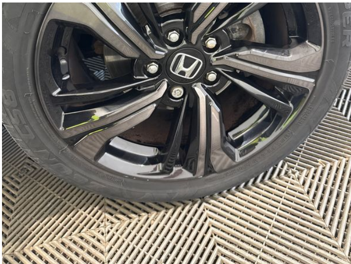
11: Wheel osf Scratched Over 50mm
