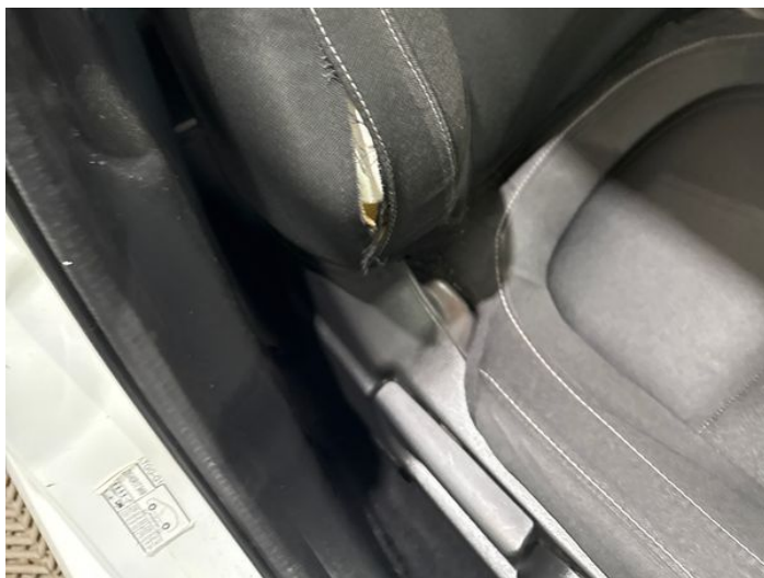
1: Seat Back Cover osf Torn Over 3mm
