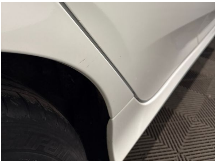
9: Door osr Chipped Edge Chip
