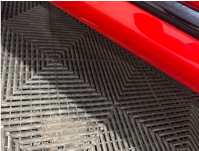
5: Sill ns Scratched Up To 25mm Thru Paint
