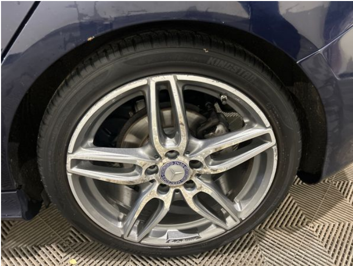
9: Wheel nsr Corroded Light
