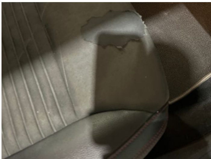
1: Seat Base Cover osr Holed Over 3mm
