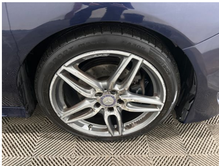
2: Wheel osf Corroded Light
