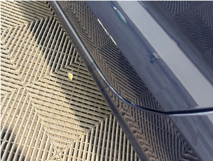
9: Door nsf Scratched Over 25mm Thru Paint
