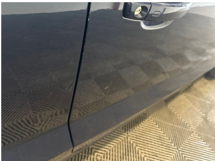
3: Door osf Chipped Edge Chip
