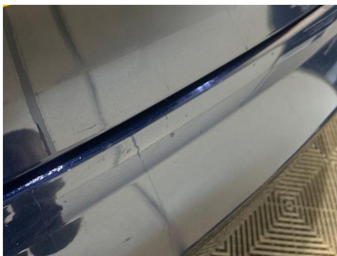
6: Tailgate Poor Previous Repair Poor Paint
