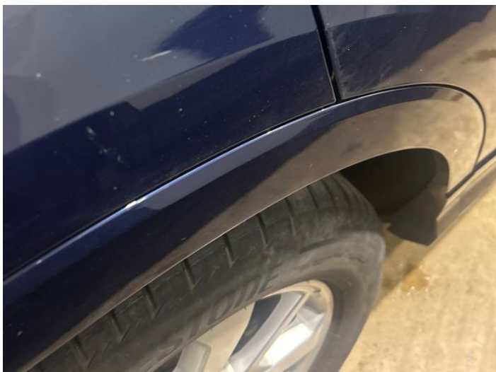
3: Qtr Panel osr Chipped 1 To 5
