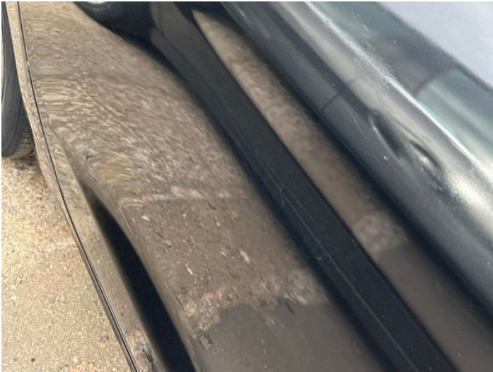
3: Door osr Poor Previous Repair Poor Paint
