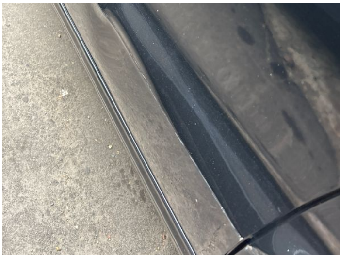
9: Door nsf Dented With Paint Damage
