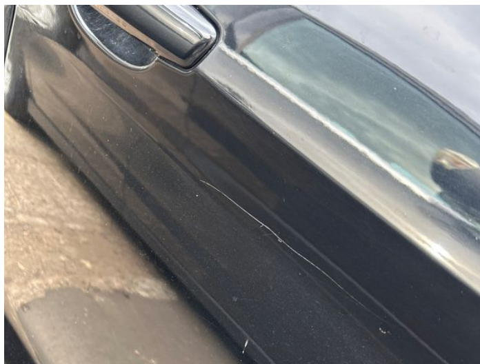
2: Door osf Scratched Over 25mm Thru Paint
