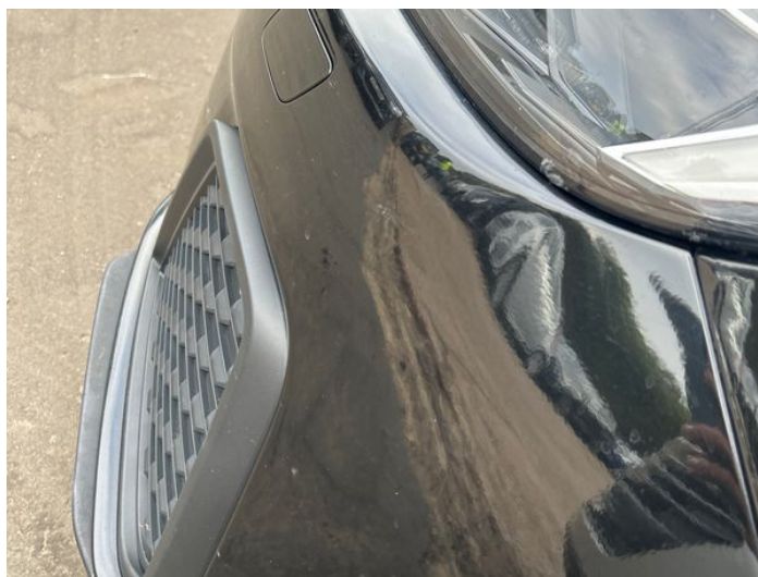
12: Bumper Front Poor Previous Repair Poor Paint
