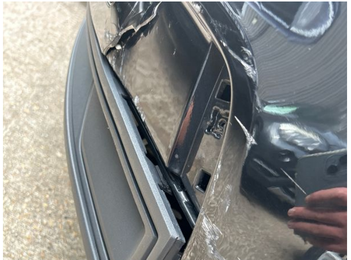
6: Bumper Rear Moulding Broken Replace
