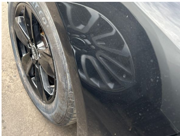
10: Wing nsf Poor Previous Repair Poor Paint
