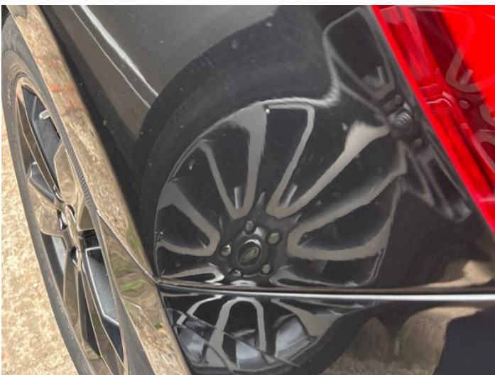
7: Qtr Panel nsr Poor Previous Repair Poor Paint
