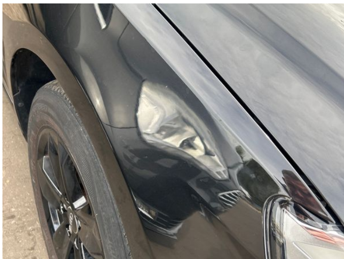
1: Wing osf Poor Previous Repair Poor Paint
