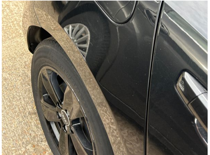
4: Qtr Panel osr Poor Previous Repair Poor Paint
