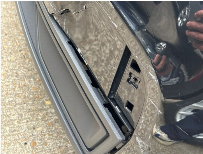
5: Bumper Rear Cracked Over 25mm
