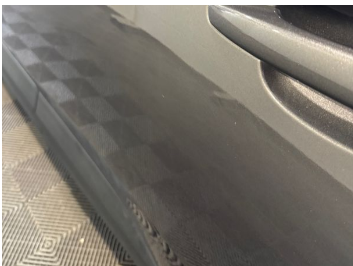
5: Door nsr Dented With Paint Damage
