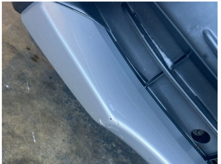
12: Bumper Front Moulding Scratched (Painted) UpTo 25mm Thru Paint
