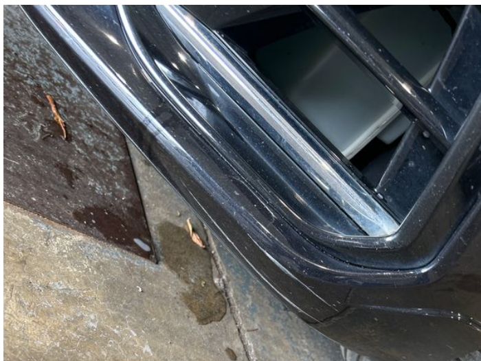
9: Bumper Front Scratched Over 100mm Thru Paint
