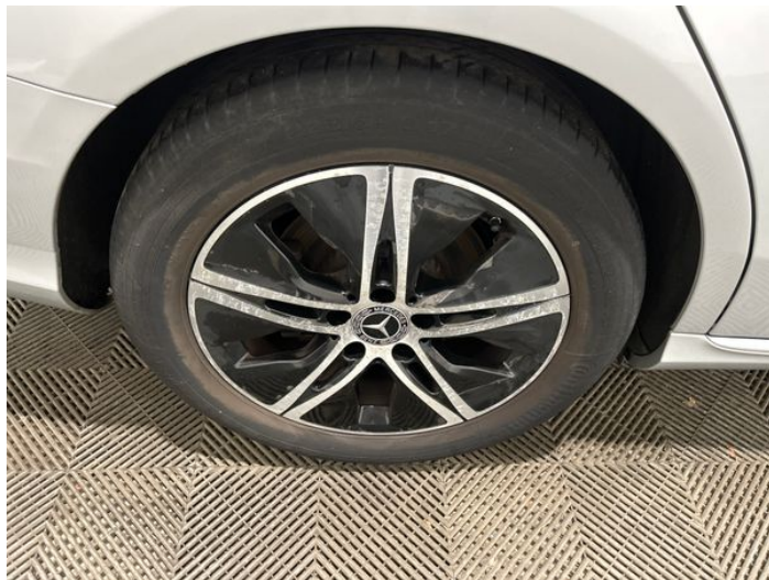
4: Wheel osr Corroded Light
