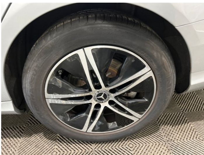
7: Wheel nsr Corroded Light
