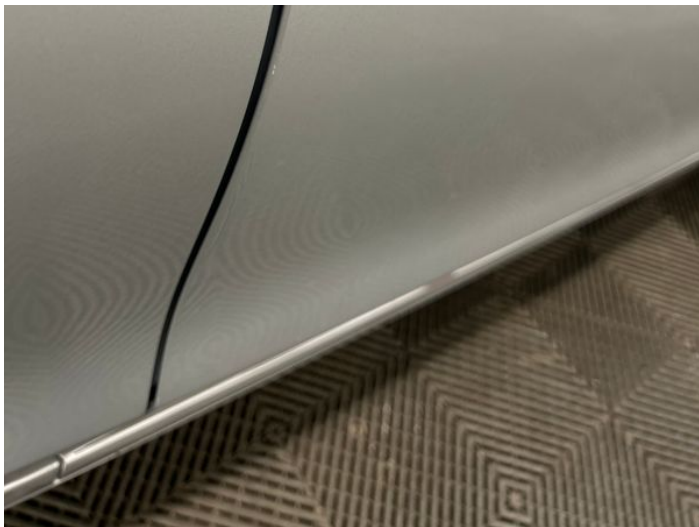
3: Door osf Chipped Edge Chip
