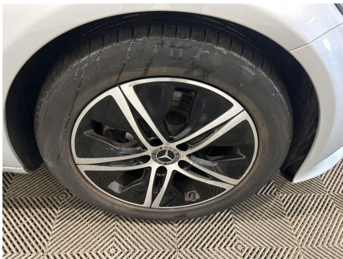
1: Wheel osf Corroded Light
