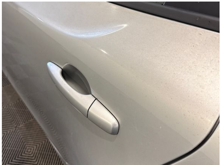
6: Door nsr Poor Previous Repair Poor Paint
