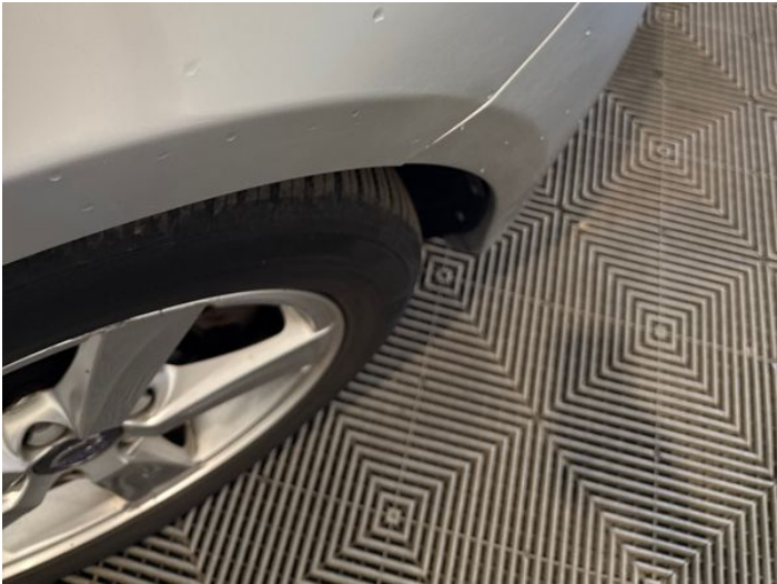
15: Wing osf Poor Previous Repair Poor Paint
