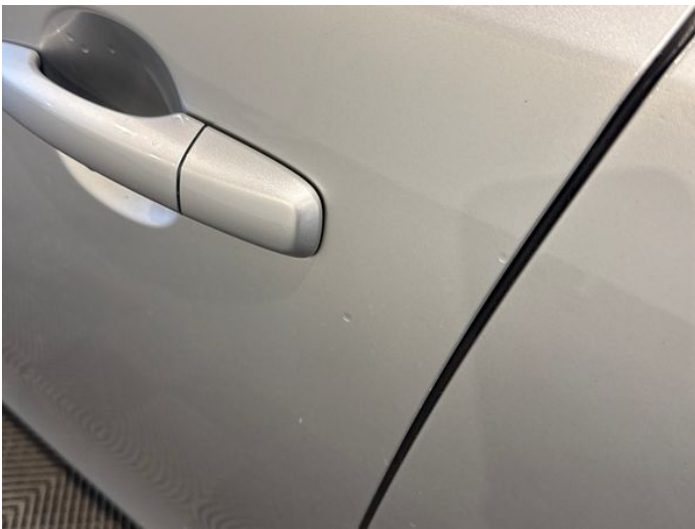
5: Door nsf Chipped 1 To 5
