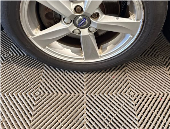
3: Wheel nsf Scratched Over 50mm
