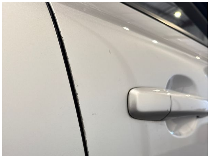
14: Door osf Chipped Edge Chip
