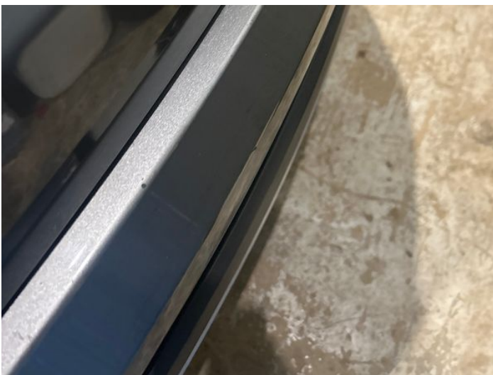
7: Bumper Rear Chipped Multiple Chips
