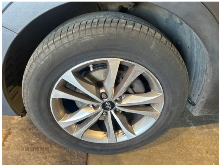
10: Wheel nsf Corroded Light
