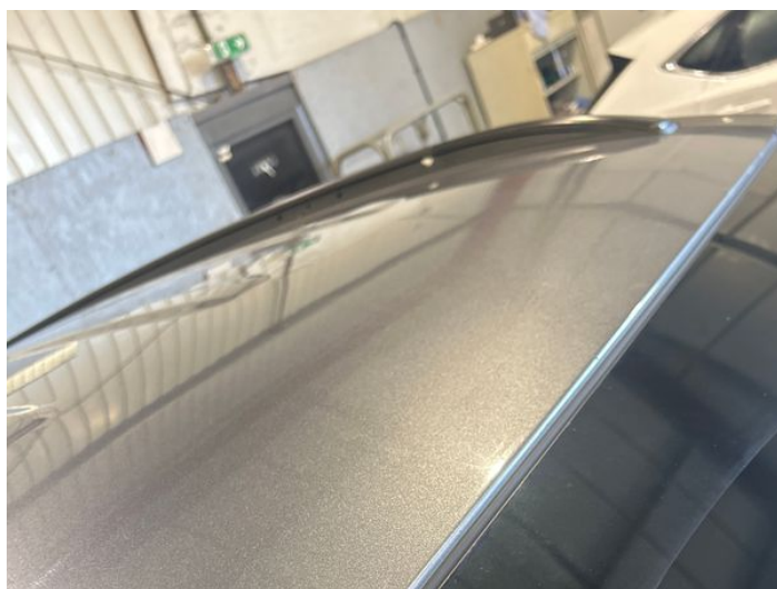
14: Roof Dented With Paint Damage
