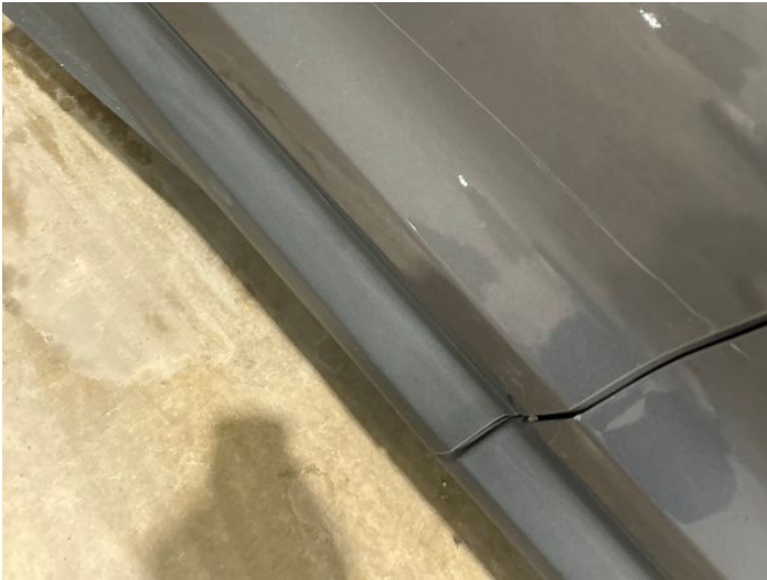
3: Door osr Scratched Over 25mm Thru Paint
