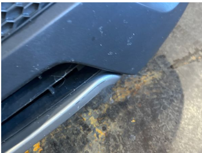
11: Bumper Front Moulding Scratched (Painted) Over 25mm Thru Paint
