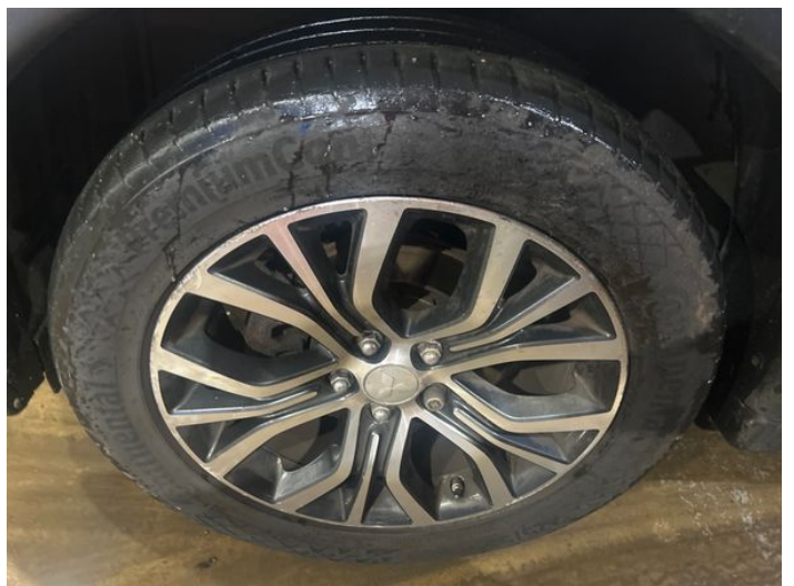
8: Wheel nsf Scratched Over 50mm
