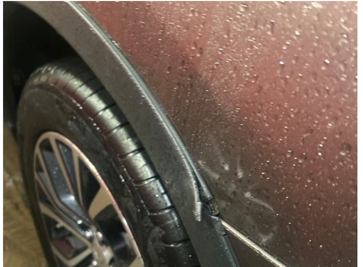
4: Qtr Panel Trim ns Broken Replace
