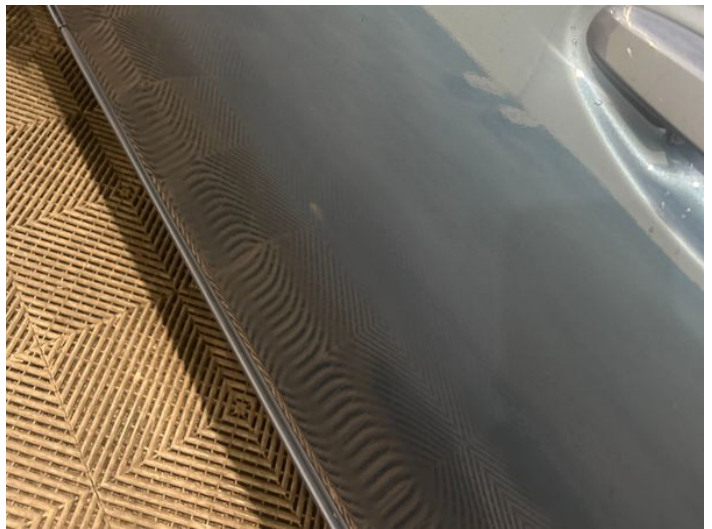
12: Door nsf Poor Previous Repair Poor Paint
