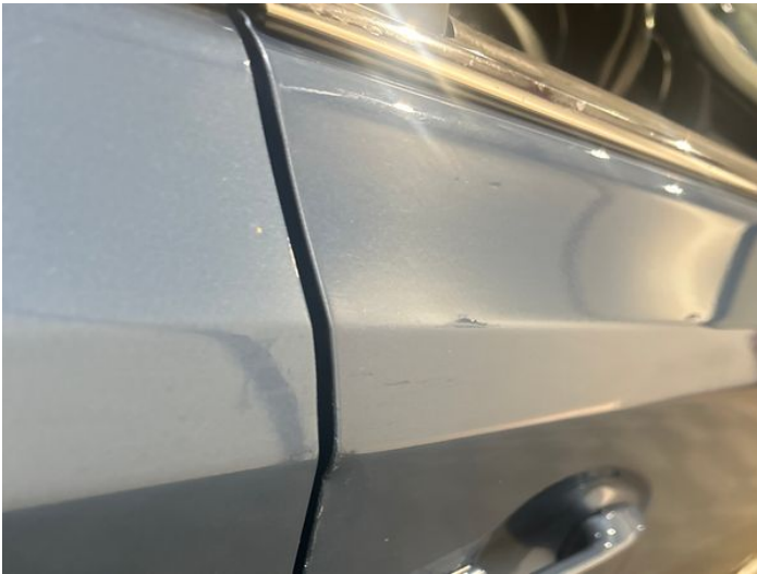
5: Door osf Dented Between 10mm + 30mm
