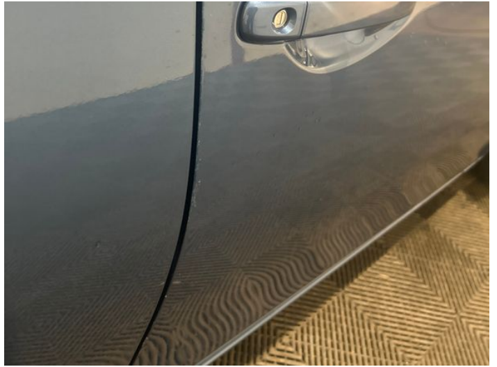
4: Door osf Chipped Edge Chip
