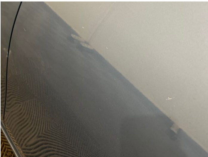
11: Door nsr Chipped 1 To 5
