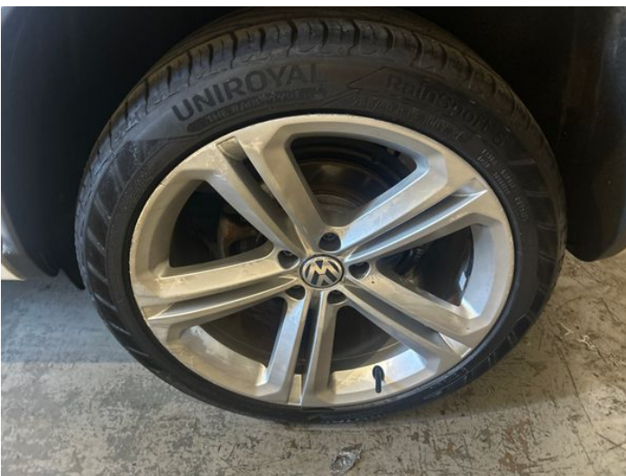
7: Wheel nsr Scratched Over 50mm
