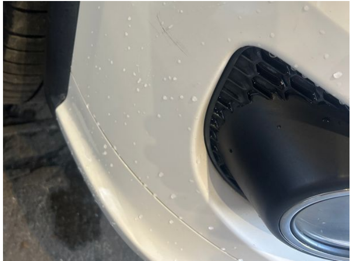
10: Bumper Front Scratched UpTo 25mm Thru Paint
