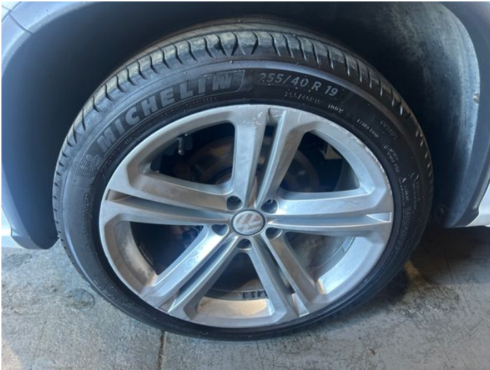
9: Wheel nsf Scratched Over 50mm
