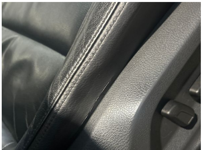
14: Seat Base Cover osf Torn Over 3mm
