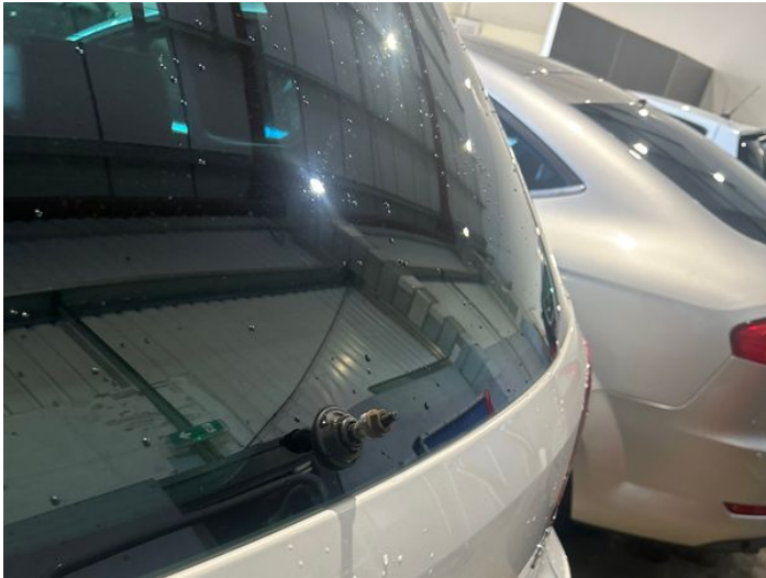
16: Wiper Rear Missing Replace
