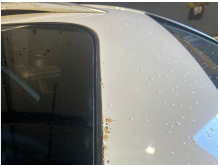
13: Roof Rusted Over 5mm
