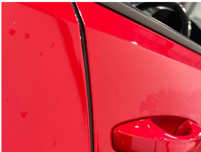
1: Door osf Chipped Edge Chip
