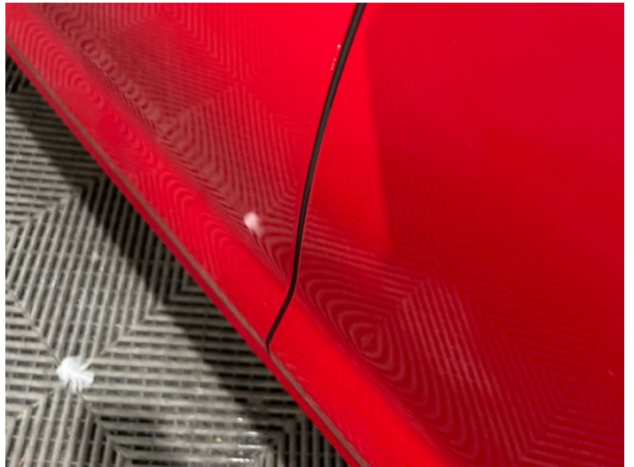
6: Door nsf Chipped Edge Chip
