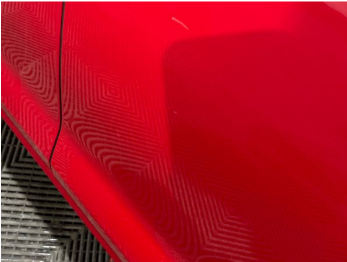
5: Door nsr Scratched UpTo 25mm Thru Paint
