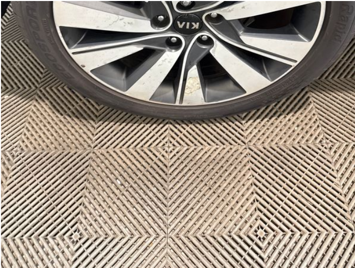
15: Wheel osr Scratched Over 50mm
