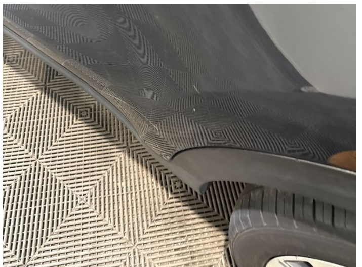
8: Door nsr Scratched Over 25mm Thru Paint
