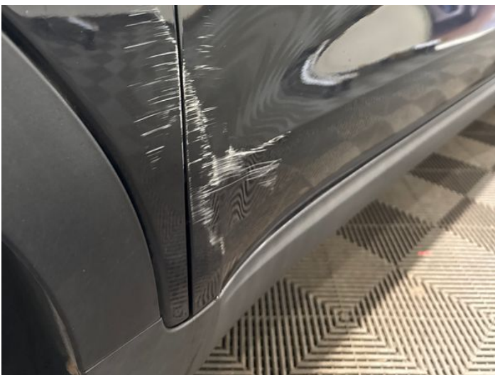
7: Door nsf Dented With Paint Damage
