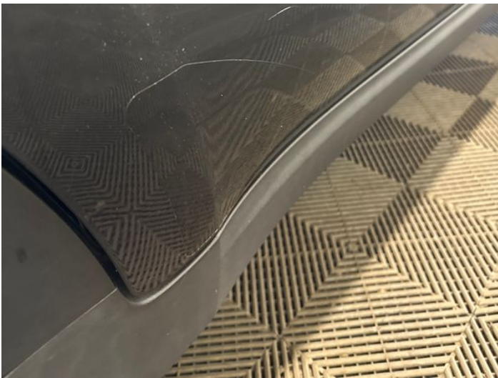
17: Door osr Scratched UpTo 25mm Thru Paint
