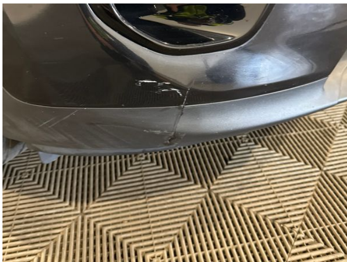
1: Bumper Front Cracked UpTo 25mm
