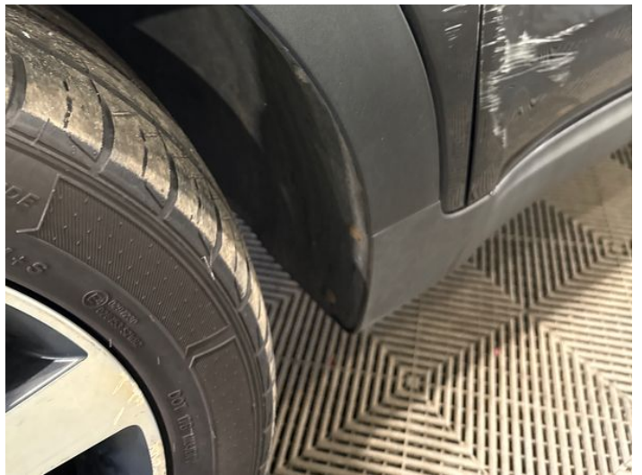
6: Wing nsf Scratched Over 25mm Thru Paint
