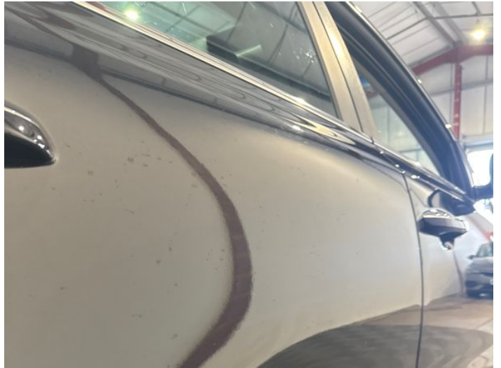
16: Door osr Dented Over 30mm
