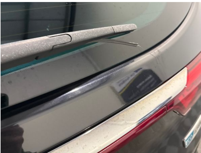
13: Wiper Rear Broken Replace
