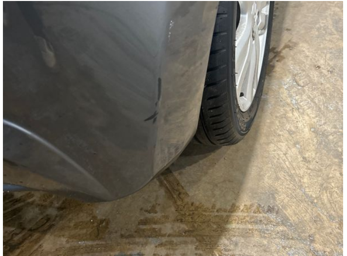
4: Bumper Rear Scratched 25 to 100mm Thru Paint
