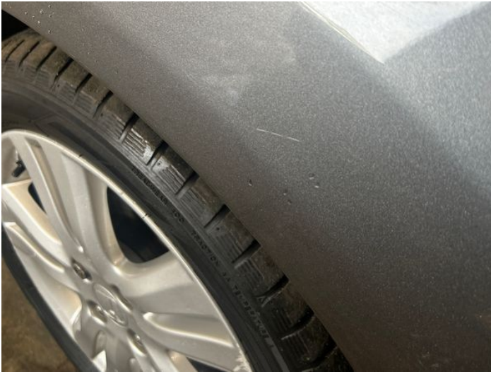
9: Wing nsf Scratched UpTo 25mm Thru Paint
