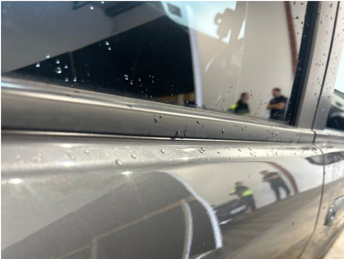
3: Door osr Dented Between 10mm + 30mm
