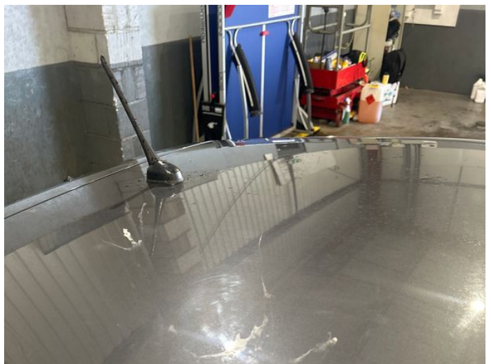
14: Roof Poor Previous Repair Poor Paint
