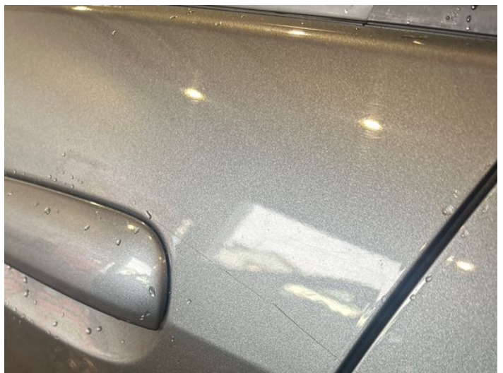
8: Door nsf Scratched Over 25mm Thru Paint
