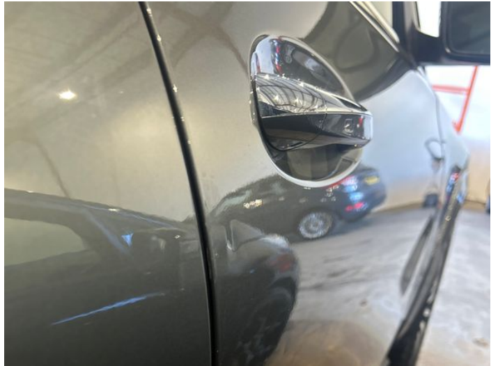
4: Door osf Dented Between 10mm + 30mm
