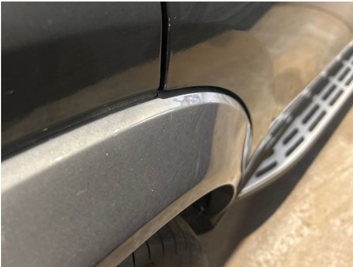
5: Door osr Chipped Edge Chip
