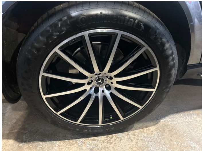
6: Wheel osr Scratched Over 50mm
