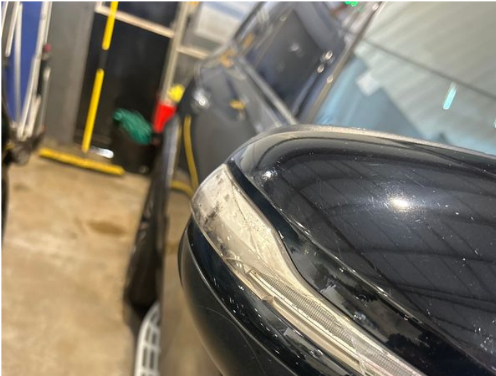
3: Door Mirror Assy osf Broken Replace
