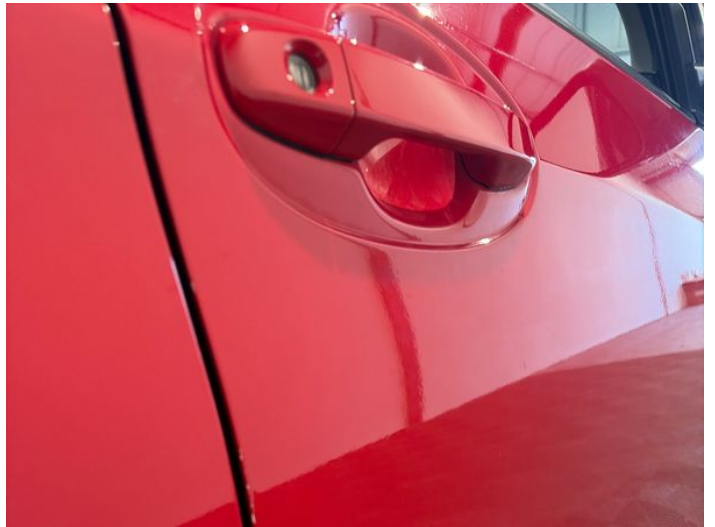
12: Door osf Chipped Edge Chip
