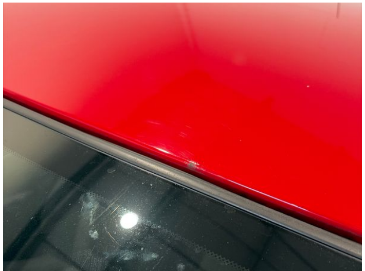
16: Roof Chipped Over 5mm
