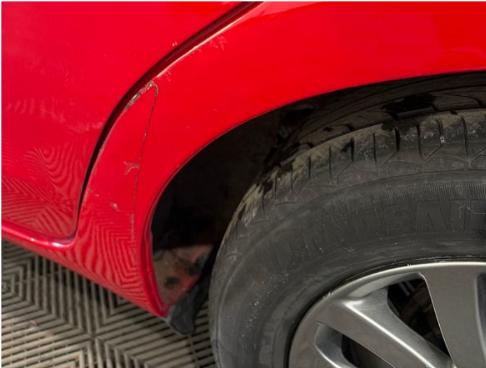
9: C Post ns Dented With Paint Damage
