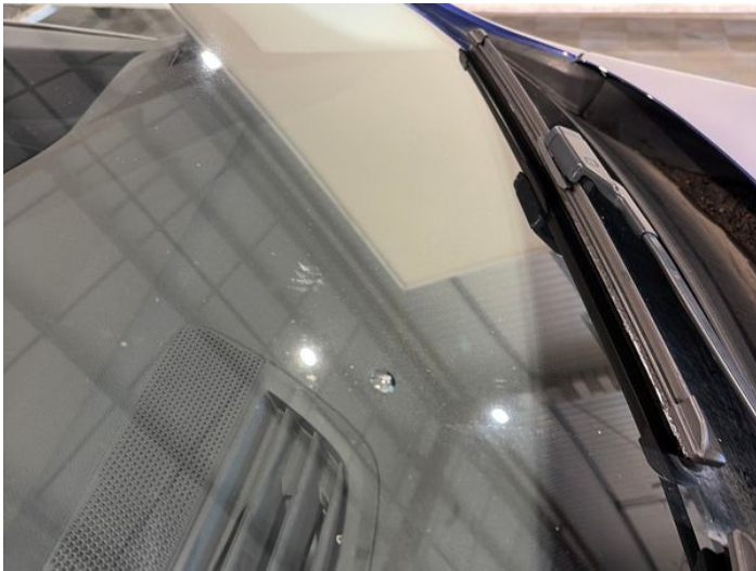
18: Screen Front Chipped Over 10mm
