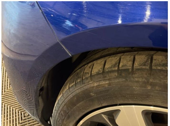
4: Wing nsf Scratched UpTo 25mm Thru Paint
