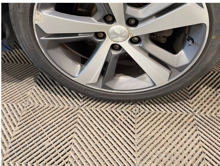
7: Wheel nsr Scratched Over 50mm
