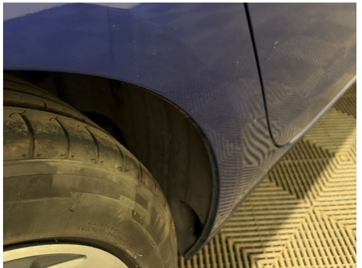
12: Qtr Panel osr Dented Between 10mm + 30mm
