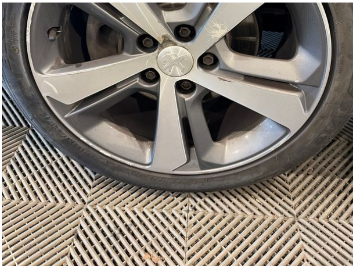
3: Wheel nsf Scratched Over 50mm
