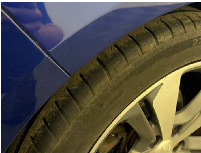
13: Qtr Panel osr Scratched UpTo 25mm Thru Paint
