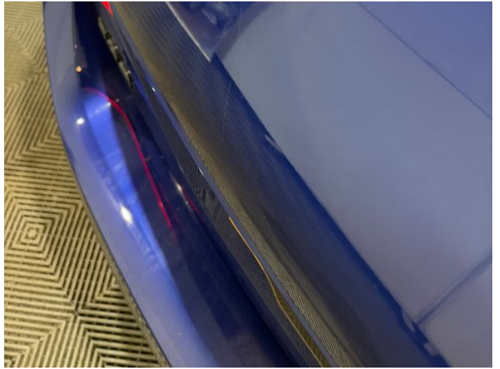
10: Tailgate Scratched Over 25mm Thru Paint
