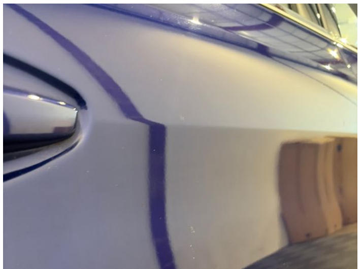
14: Door osr Scratched Over 25mm Thru Paint
