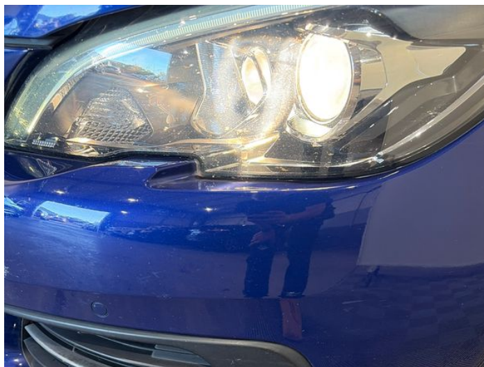
2: Bumper Front Scratched 25 to 100mm Thru Paint
