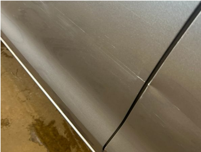
9: Door nsf Dented With Paint Damage
