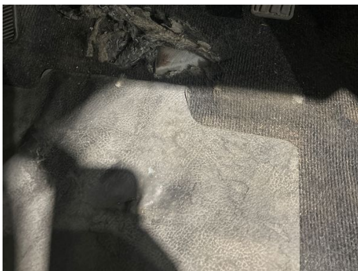
1: Carpets Front Torn Over 10mm
