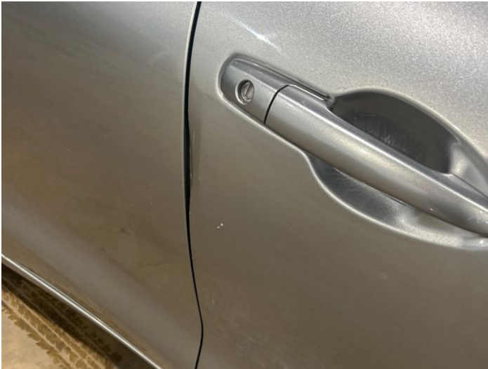
3: Door osf Dented With Paint Damage
