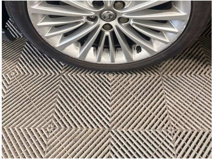
4: Wheel nsf Scratched Over 50mm
