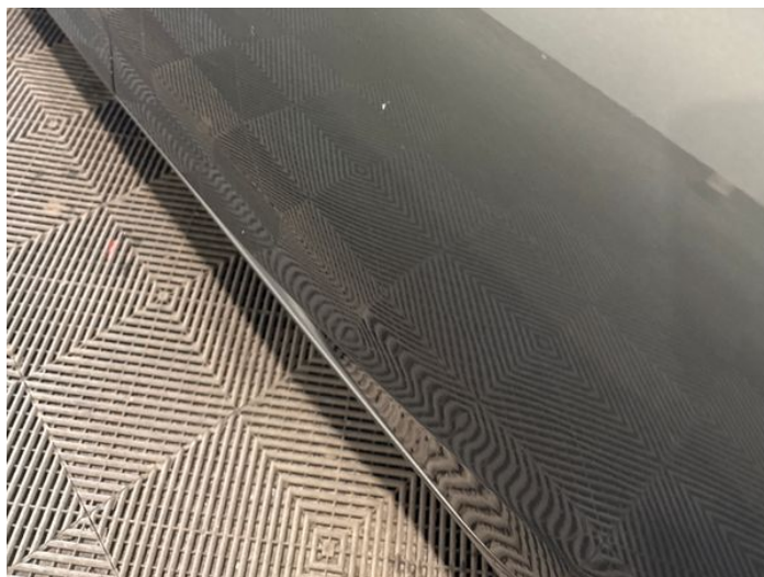
10: Door nsr Scratched Over 25mm Thru Paint
