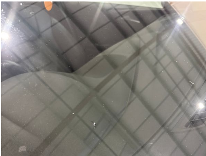
21: Screen Front Chipped UpTo 10mm
