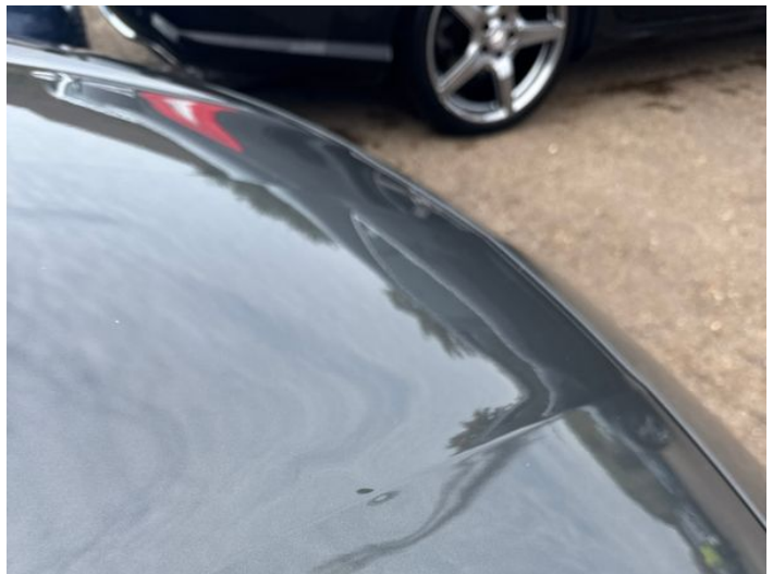
22: Bonnet Dented Between 10mm + 30mm
