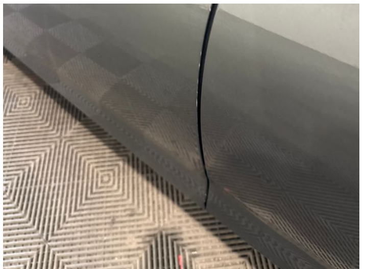
8: Door nsf Chipped Edge Chip
