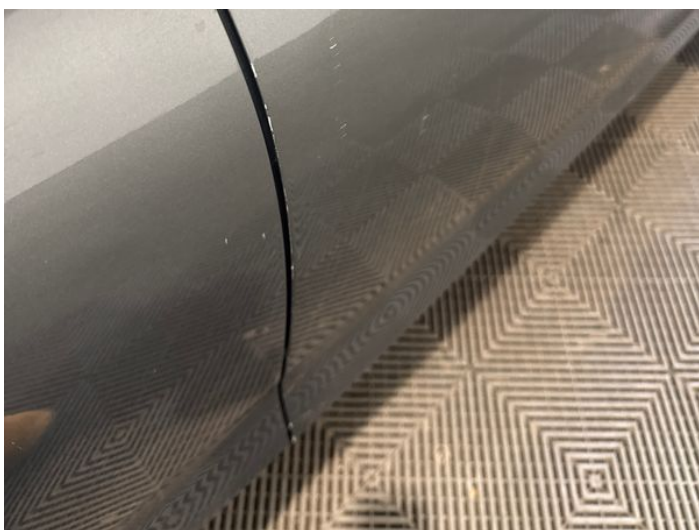
19: Door osf Dented With Paint Damage
