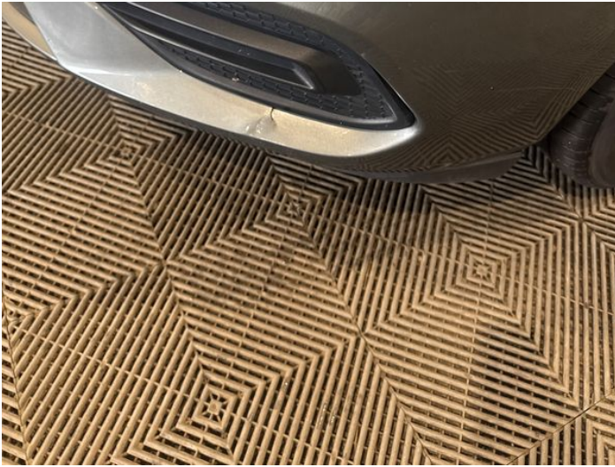
3: Bumper Front Cracked UpTo 25mm
