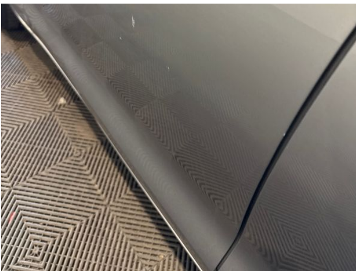
7: Door nsf Dented With Paint Damage
