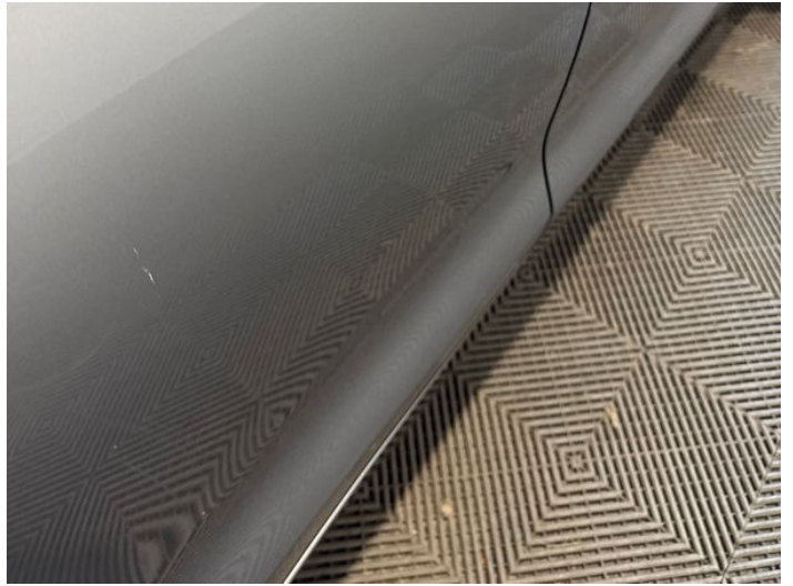
16: Door osr Dented Between 10mm + 30mm
