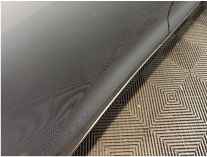
17: Door osr Scratched Over 25mm Thru Paint
