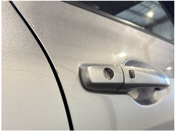
18: Door osf Chipped Edge Chip
