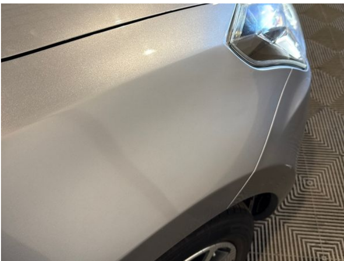
19: Wing osf Poor Previous Repair Poor Paint
