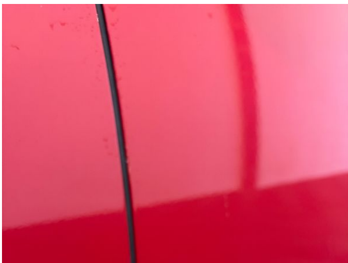
17: Door osf Chipped Edge Chip
