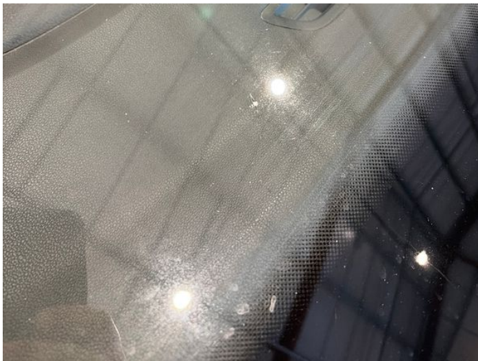
21: Screen Front Chipped Over 10mm
