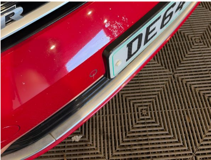
5: Bumper Front Poor Previous Repair Paint Flake
