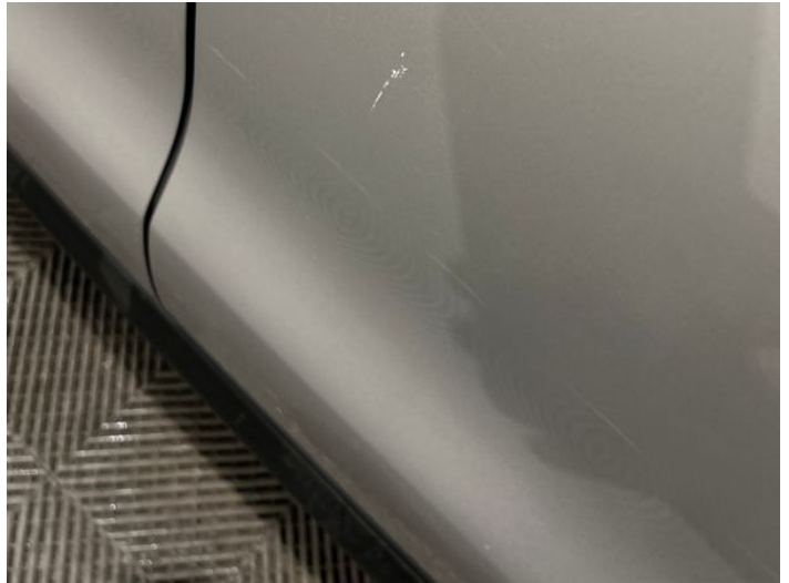
10: Door nsr Scratched UpTo 25mm Thru Paint
