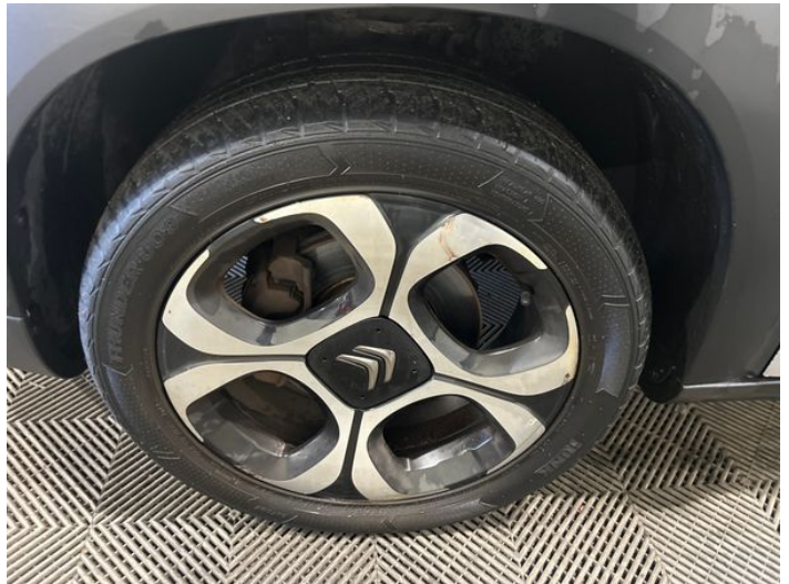
12: Wheel nsf Scratched Over 50mm
