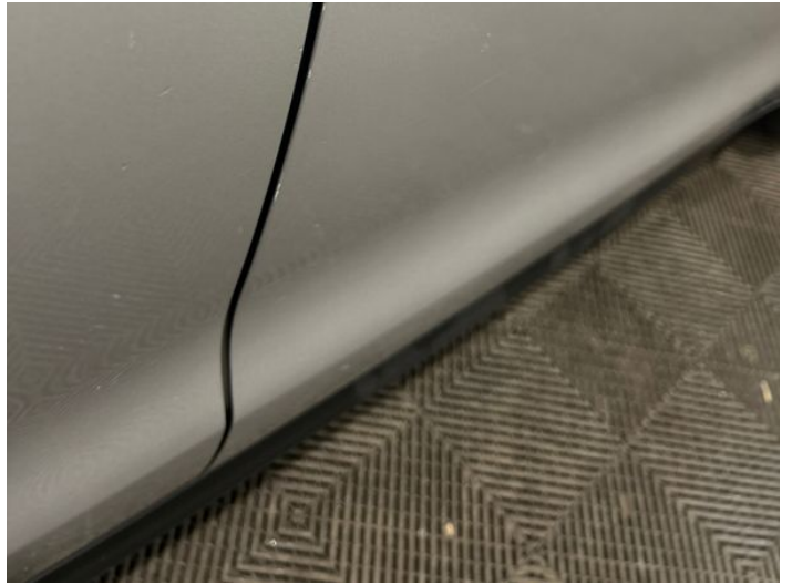
4: Door osf Chipped Edge Chip
