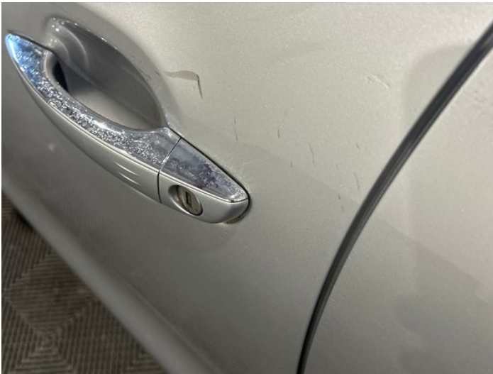
11: Door nsf Scratched Over 25mm Thru Paint
