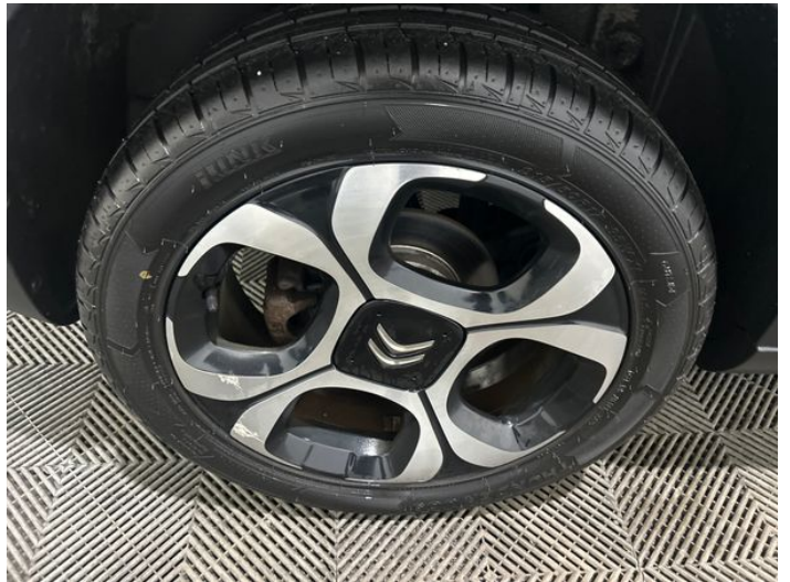
6: Wheel osr Corroded Light
