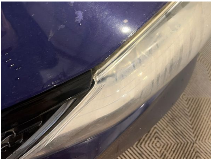
15: Bonnet Poor Previous Repair Paint Flake
