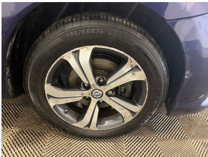
1: Wheel osf Corroded Light
