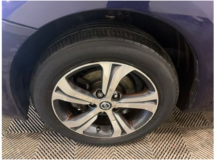
4: Wheel nsf Corroded Light
