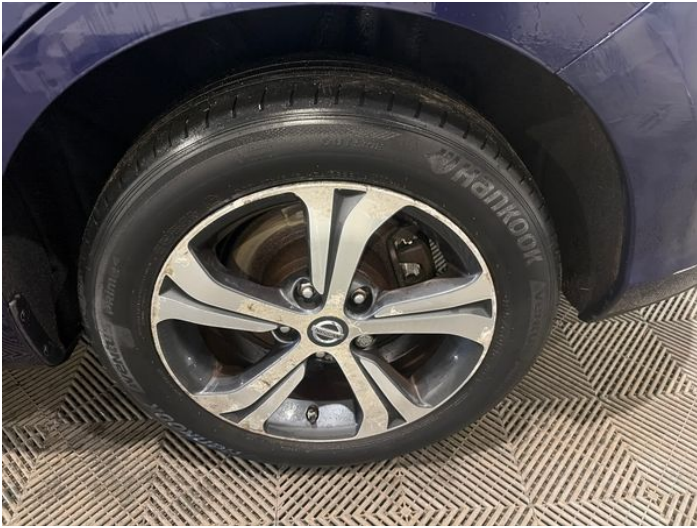
3: Wheel nsr Corroded Light
