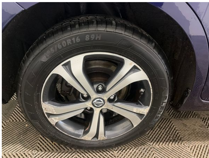
2: Wheel osr Corroded Light
