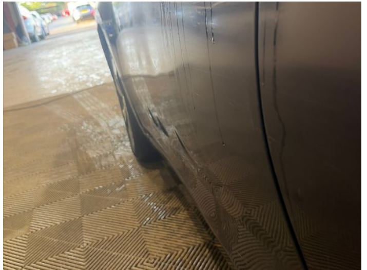
12: Door nsf Dented Over 30% Of Panel
