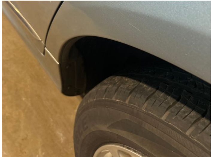
10: Qtr Panel nsr Dented Between 10mm + 30mm
