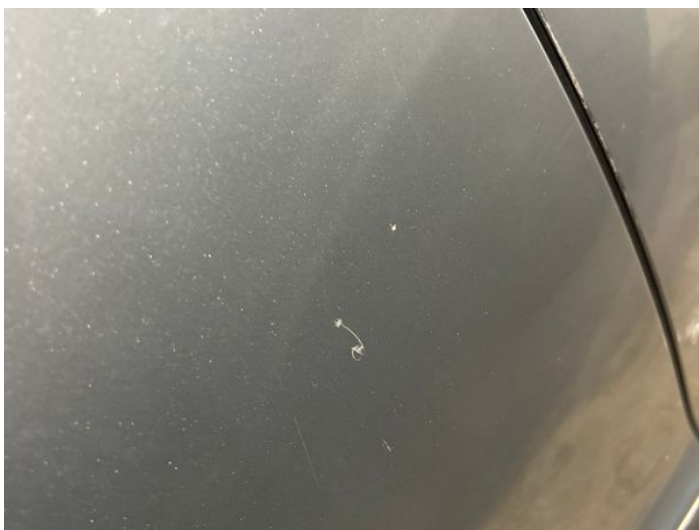
5: Door osr Scratched UpTo 25mm Thru Paint
