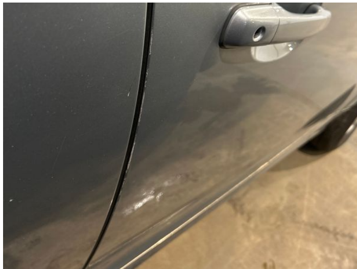
4: Door osf Chipped Edge Chip
