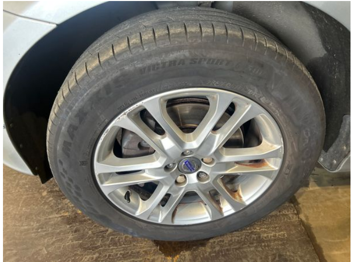
16: Wheel nsf Scratched Over 50mm
