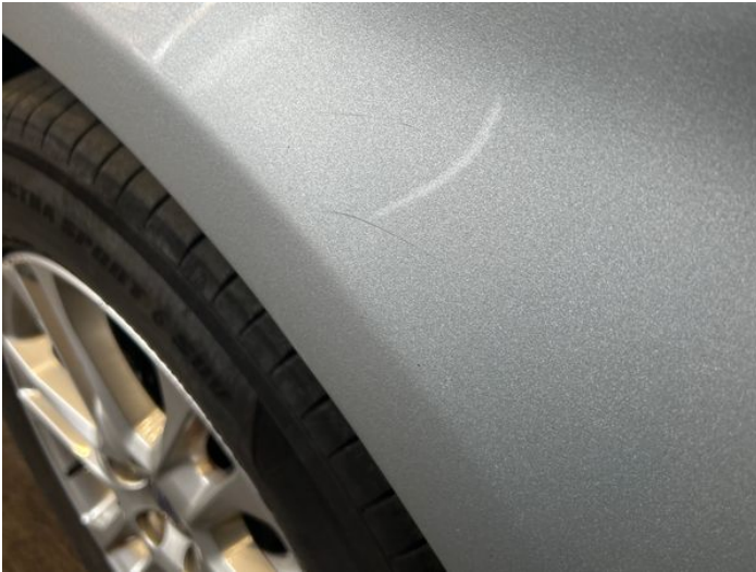
15: Wing nsf Scratched Over 25mm Thru Paint
