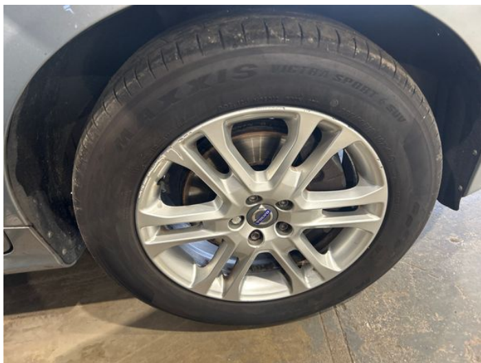
1: Wheel osf Scratched Over 50mm
