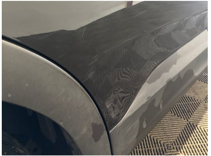
18: Door osr Dented With Paint Damage
