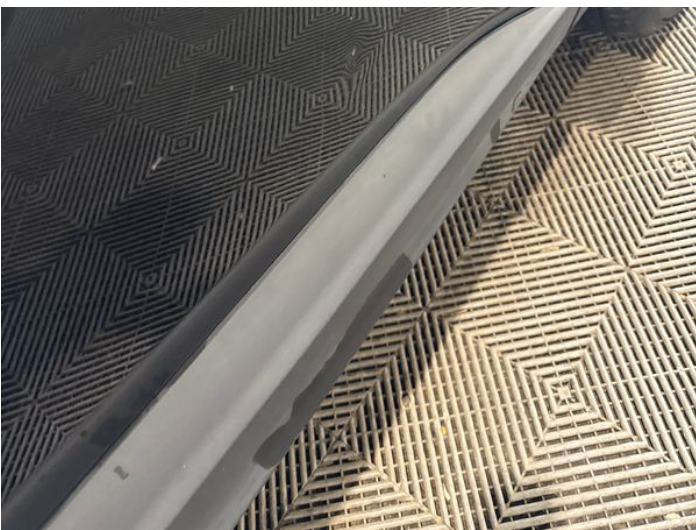
19: Door osf Dented Between 10mm + 30mm
