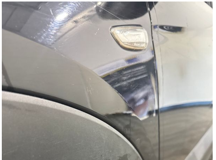
6: Wing nsf Dented Between 10mm + 30mm
