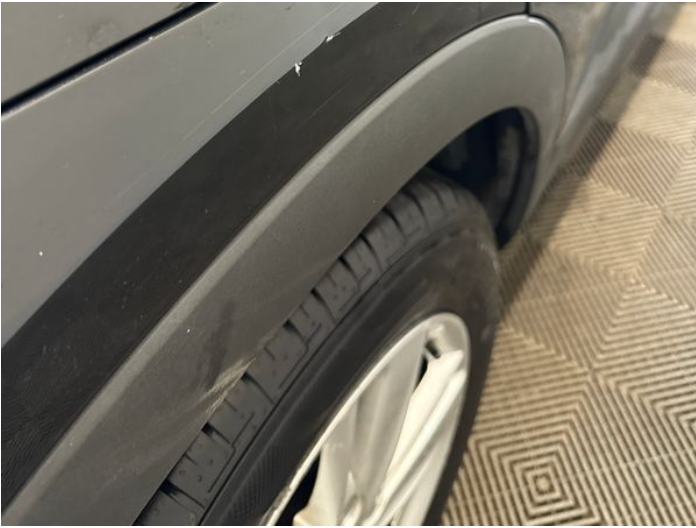
15: Qtr Panel osr Dented Between 10mm + 30mm
