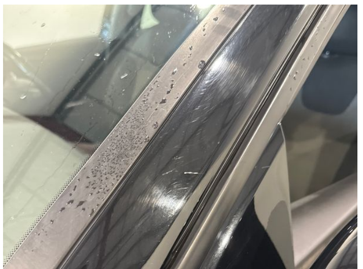
8: A Post ns Scratched UpTo 25mm Thru Paint
