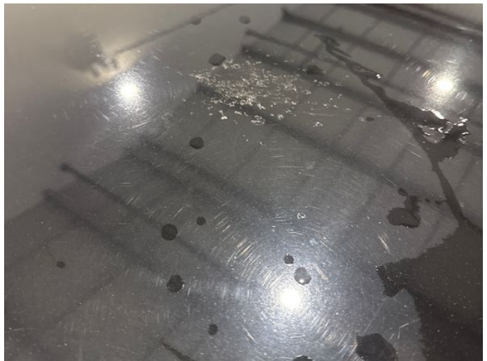
24: Roof Scratched Over 25mm Thru Paint
