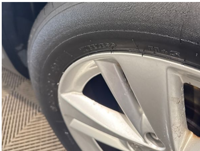
2: Tyre nsr Damaged Replace
