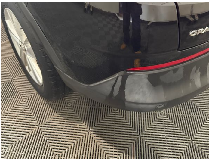
13: Bumper Rear Scratched 25 to 100mm Thru Paint
