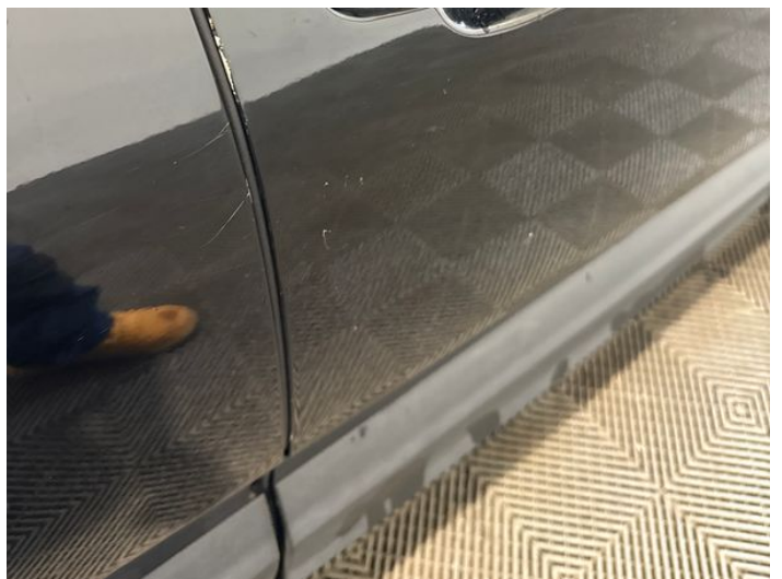
20: Door osf Scratched Over 25mm Thru Paint
