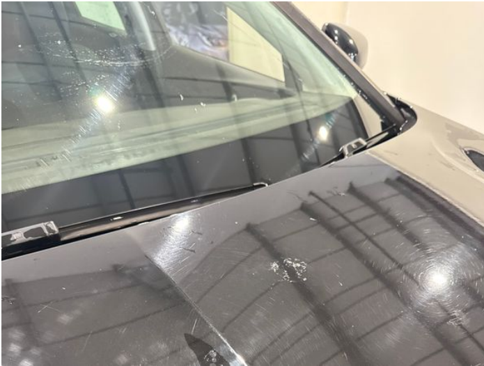
3: Bonnet Scratched Over 25mm Thru Paint
