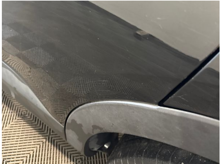
10: Door nsr Scratched Over 25mm Thru Paint
