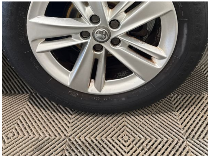
12: Wheel nsr Corroded Light
