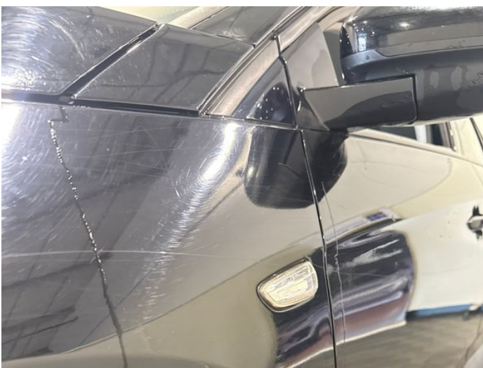
7: Wing nsf Scratched Over 25mm Thru Paint
