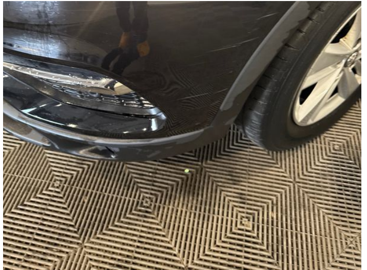
4: Bumper Front Scratched Over 100mm Thru Paint
