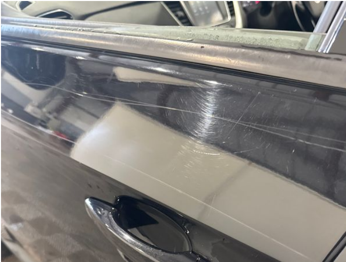
9: Door nsf Scratched Over 25mm Thru Paint
