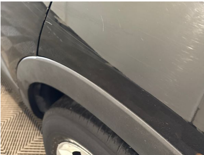
11: Qtr Panel nsr Scratched Over 25mm Thru Paint
