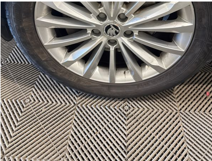
5: Wheel nsf Scratched Up To 50mm
