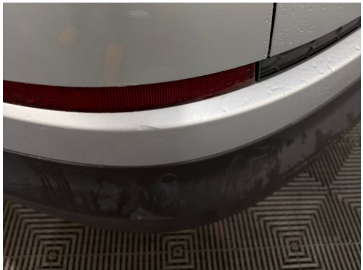
22: Bumper Rear Dented Between 10mm + 30mm
