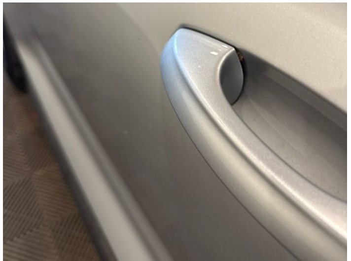
6: Door nsf Dented Between 10mm + 30mm
