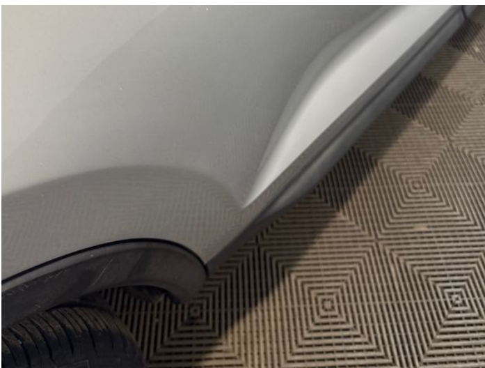
13: Door osr Dented Between 10mm + 30mm
