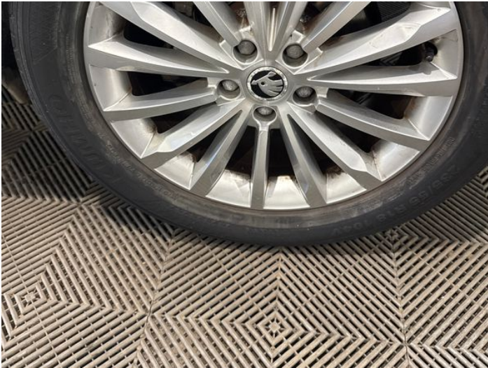
9: Wheel nsr Scratched Up To 50mm
