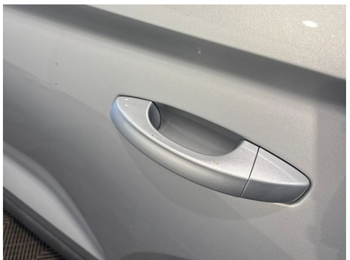
8: Door nsr Poor Previous Repair Rippled UpTo 30%
