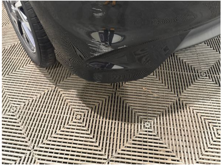
10: Bumper Rear Dented With Paint Damage
