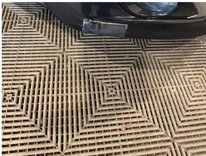
2: Bumper Front Cracked Over 25mm
