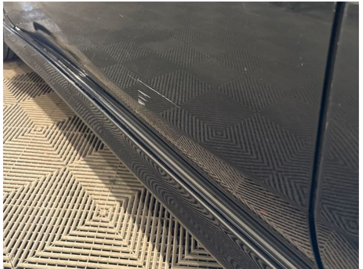
6: Door nsf Scratched Over 25mm Thru Paint
