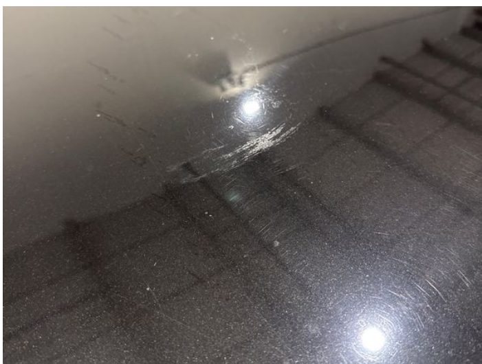
19: Roof Scratched Over 25mm Thru Paint
