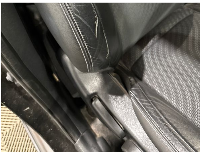
20: Seat Back Cover osf Scuffed Over 25mm
