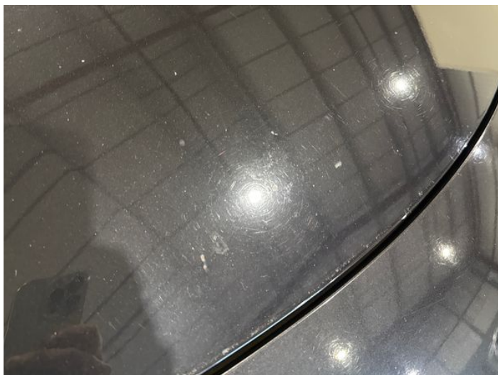
1: Bonnet Chipped Multiple Chips
