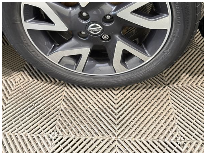
8: Wheel nsr Scratched Over 50mm
