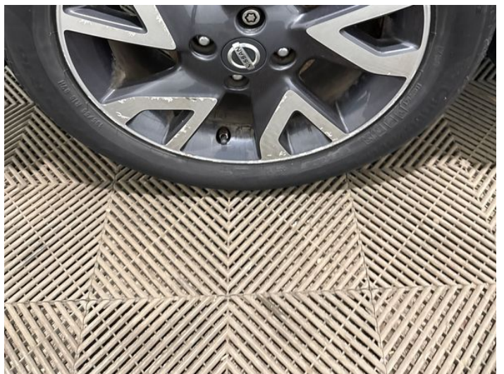
14: Wheel osr Scratched Over 50mm
