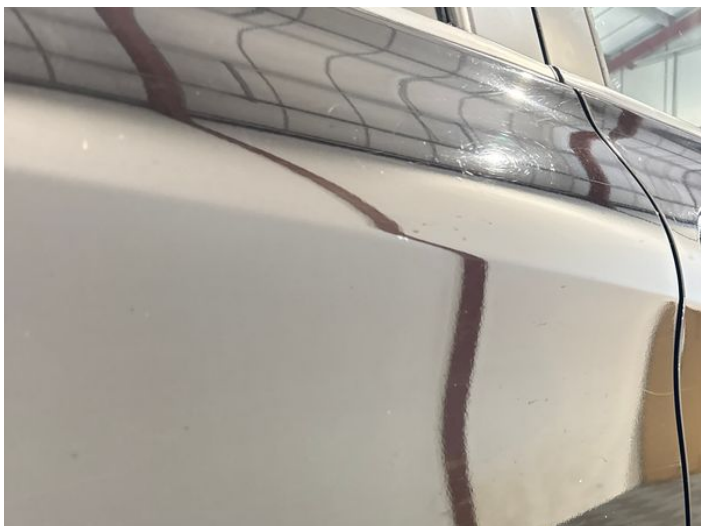
15: Door osr Scratched Over 25mm Thru Paint
