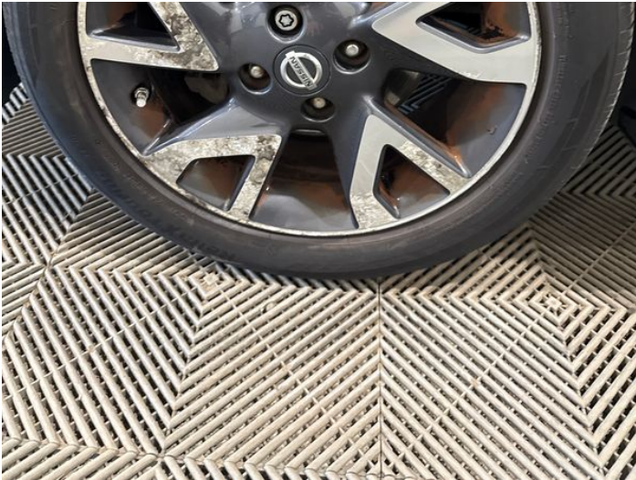
3: Wheel nsf Scratched Over 50mm
