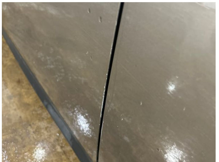
8: Door nsf Chipped Edge Chip
