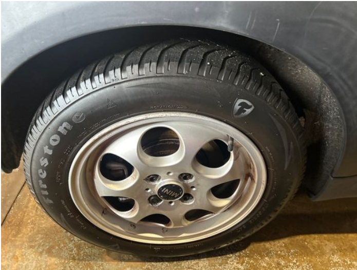
3: Wheel osr Scratched Over 50mm
