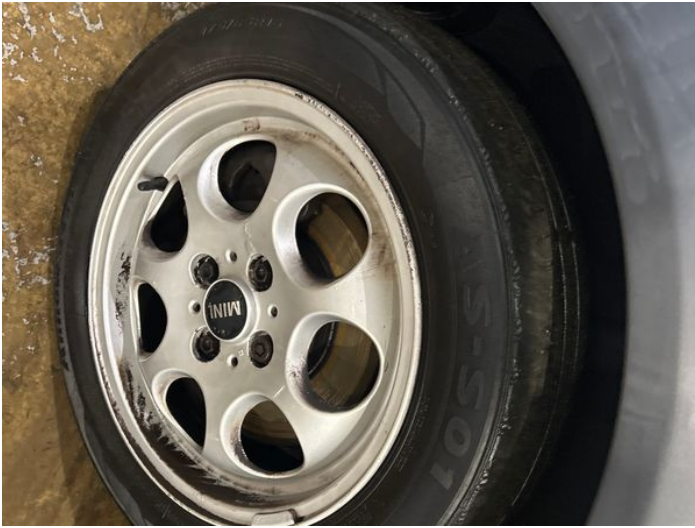
9: Wheel nsf Scratched Over 50mm
