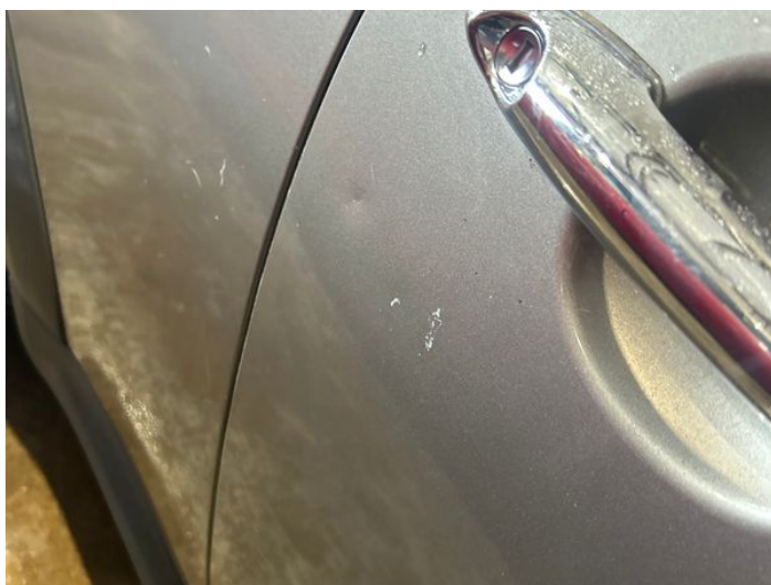
1: Door osf Dented With Paint Damage
