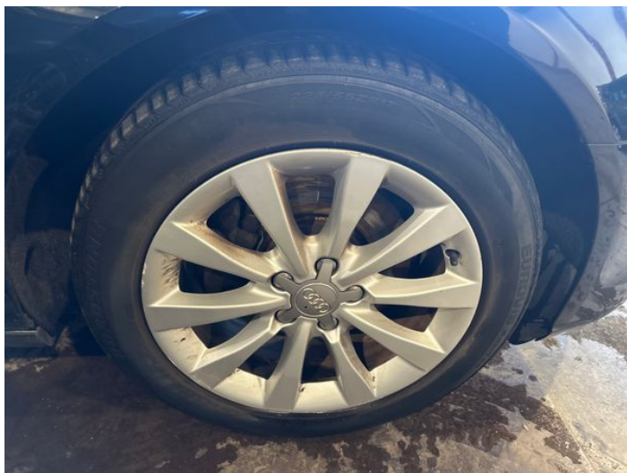
1: Wheel osf Scratched Up To 50mm
