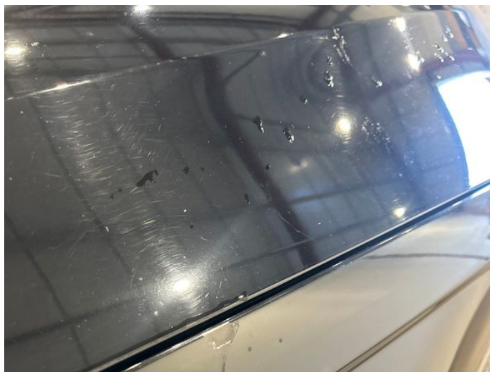
2: Wing osf Poor Previous Repair Paint Flake
