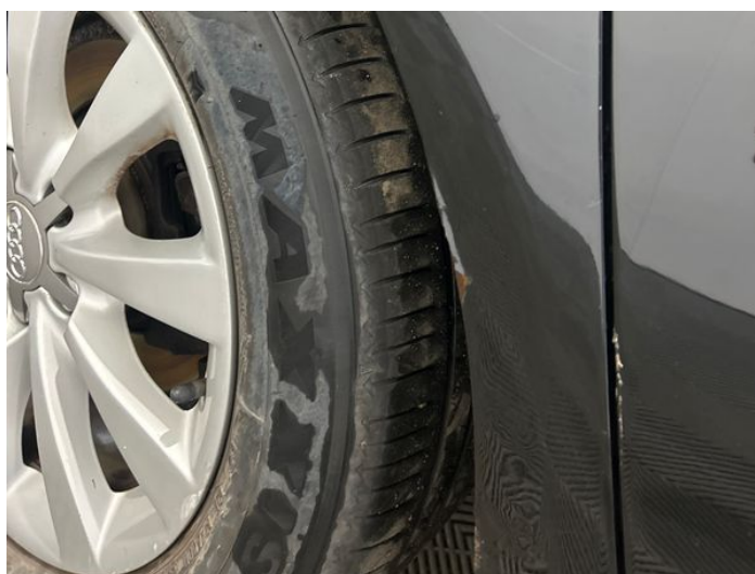
6: Qtr Panel osr Poor Previous Repair Paint Flake
