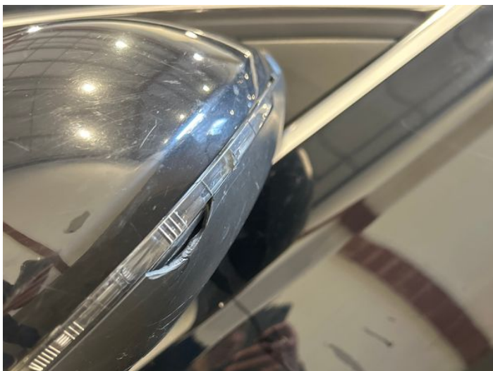
3: Door Mirror Assy osf Broken Replace
