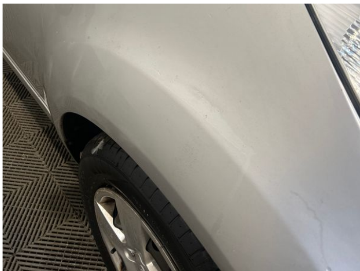
1: Wing osf Poor Previous Repair Poor Paint
