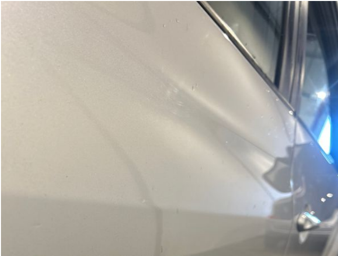
3: Door osr Dented Over 30mm
