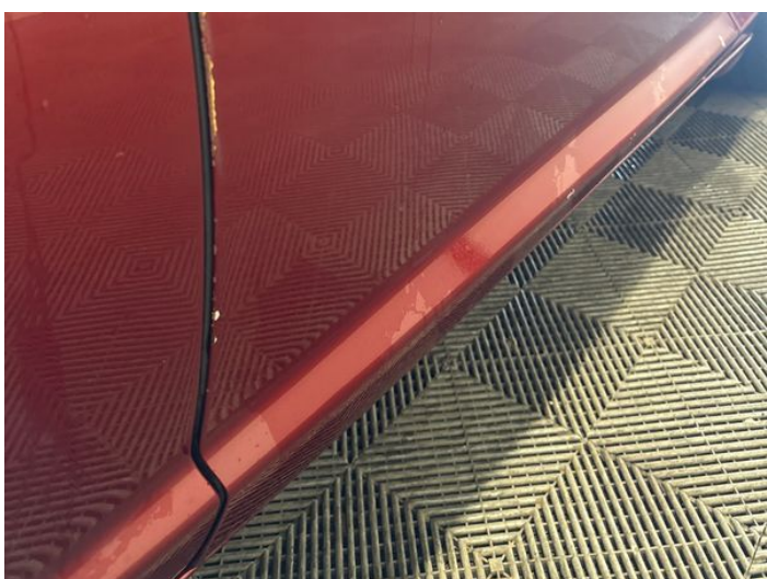
19: Door osf Dented With Paint Damage
