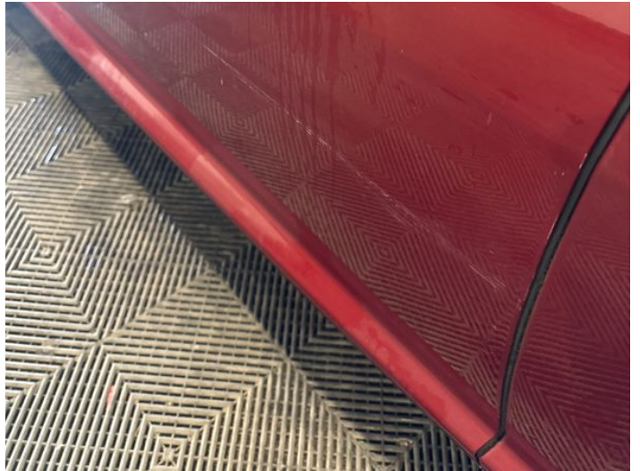
10: Door nsf Dented With Paint Damage
