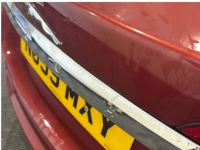
15: Boot Lid Scratched Over 25mm Thru Paint
