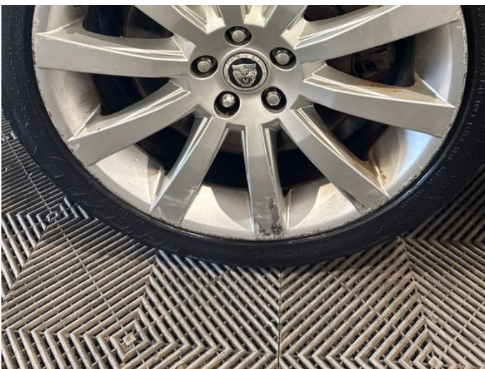
7: Wheel nsf Scratched Over 50mm
