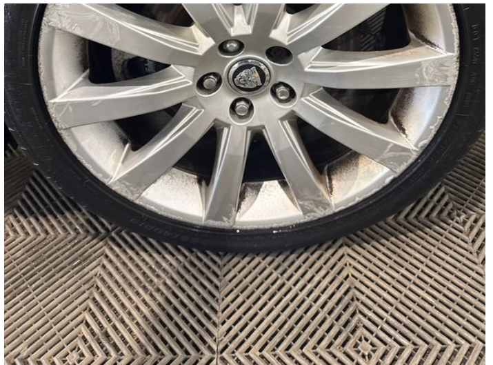
12: Wheel nsr Scratched Over 50mm
