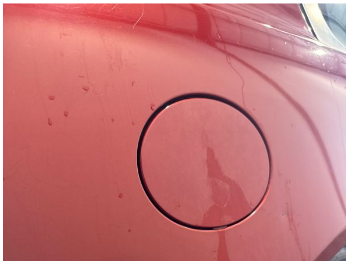
16: Qtr Panel osr Dented With Paint Damage
