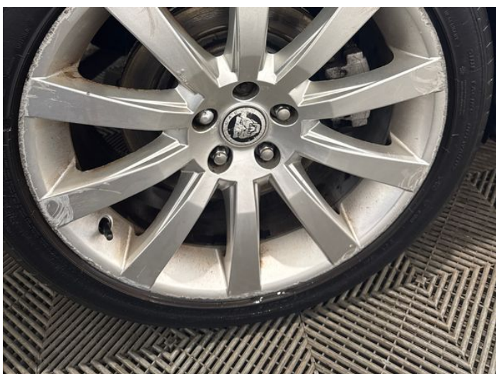
17: Wheel osr Scratched Over 50mm
