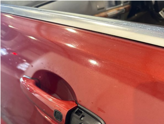
9: Handle Outer nsf Broken Replace
