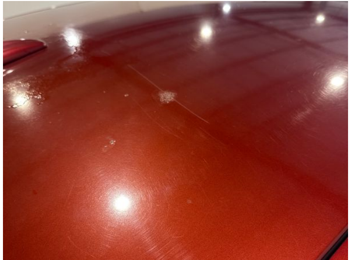
22: Roof Scratched Over 25mm Thru Paint
