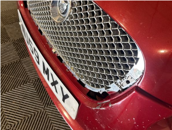
3: Bumper Front Grill Broken Replace
