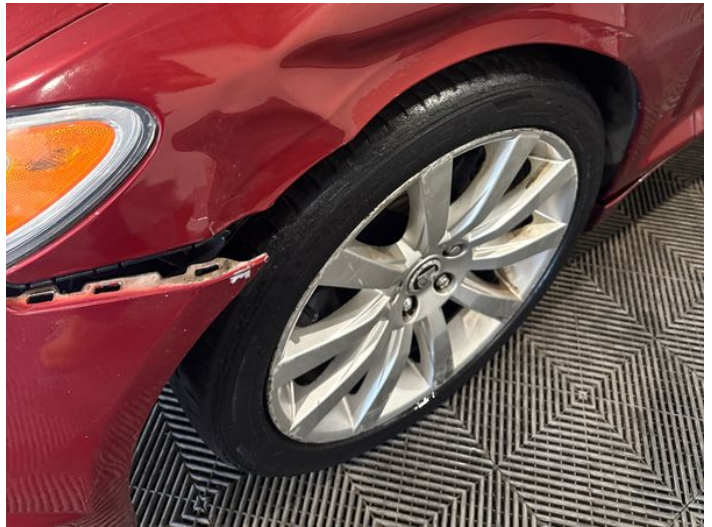
6: Wing nsf Dented Over 30% Of Panel
