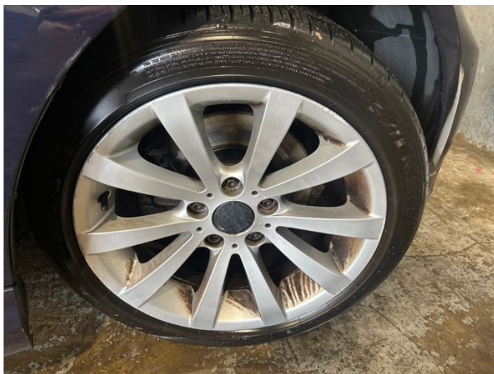
1: Wheel osf Scratched Over 50mm
