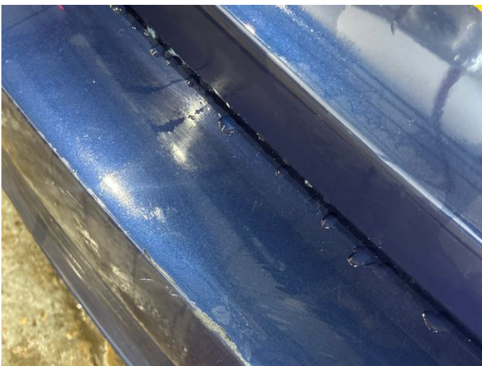
7: Bumper Rear Poor Previous Repair Paint Flake
