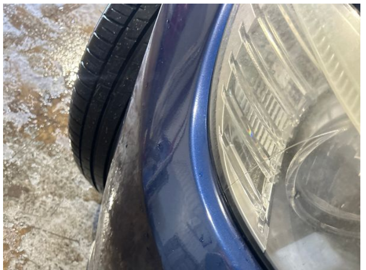
14: Bumper Front Poor Previous Repair Poor Paint
