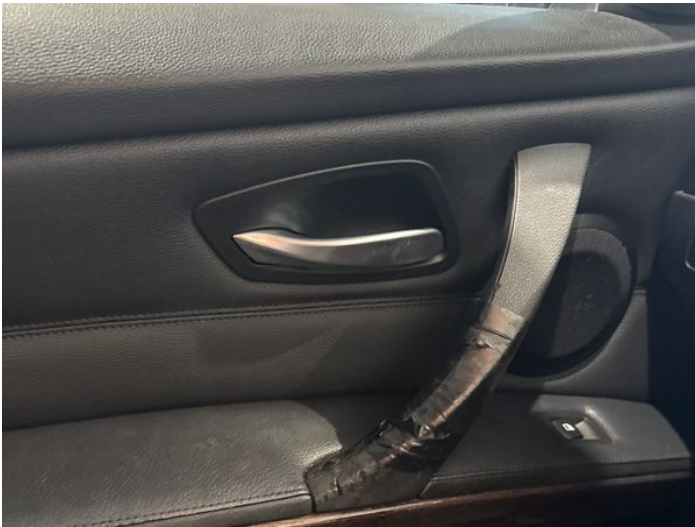
17: Door Pad nsf Scuffed Over 25mm
