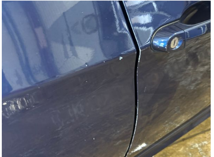
4: Door osr Chipped 1 To 5
