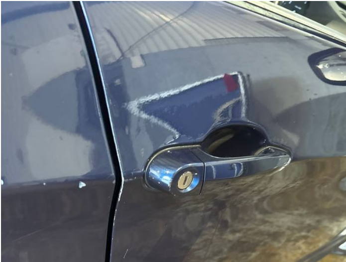
3: Door osf Chipped Edge Chip
