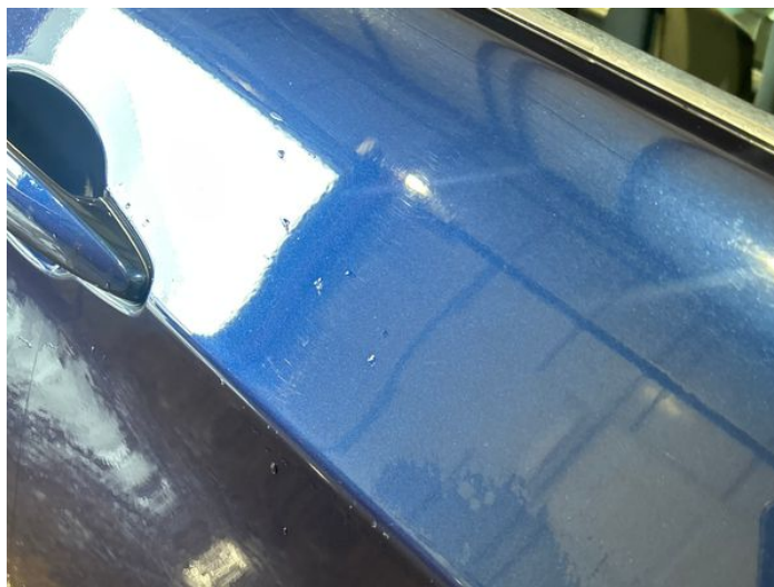
2: Door osf Chipped 1 To 5
