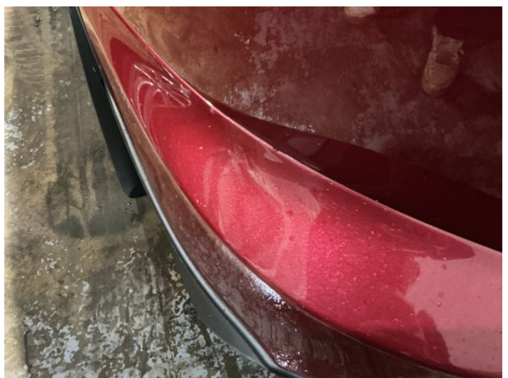
8: Qtr Panel nsr Chipped 1 To 5
