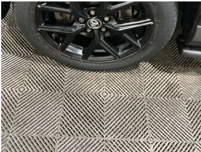
11: Wheel nsf Scratched Over 50mm
