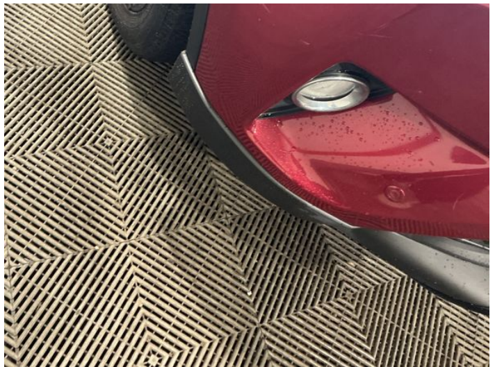
12: Bumper Front Scratched Over 100mm Thru Paint
