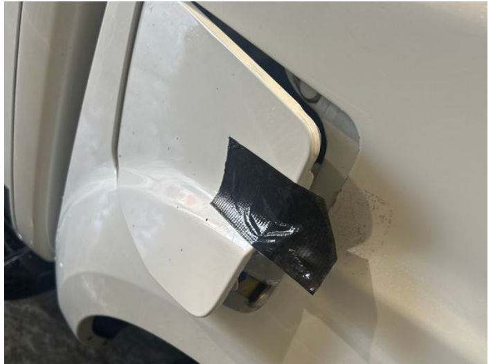
4: Fuel Flap Missing Replace
