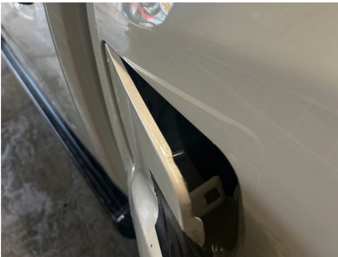
5: Qtr Panel nsr Dented Between 10mm + 30mm
