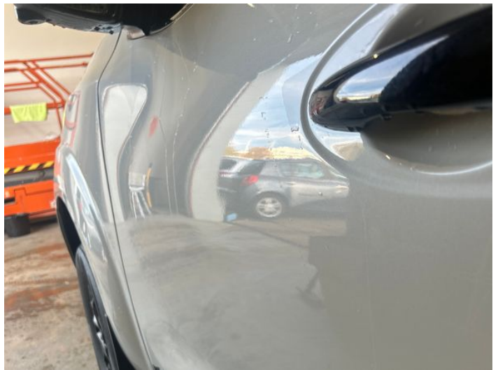
6: Door nsf Dented Over 30mm
