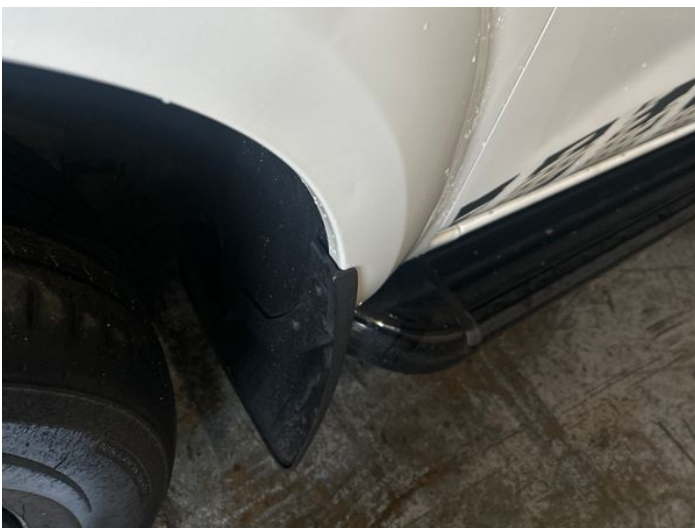
7: Wing nsf Dented Over 30mm
