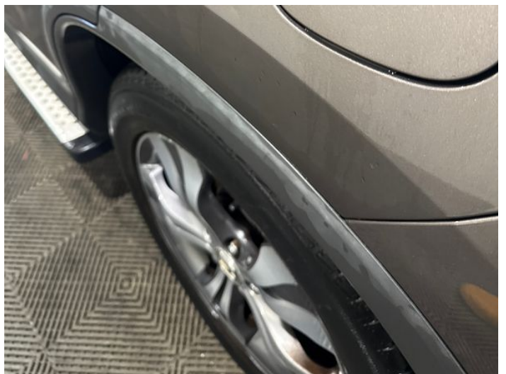
8: Qtr Panel nsr Dented Between 10mm + 30mm
