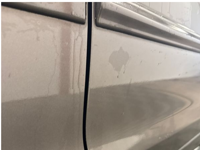
15: Door osf Chipped Edge Chip
