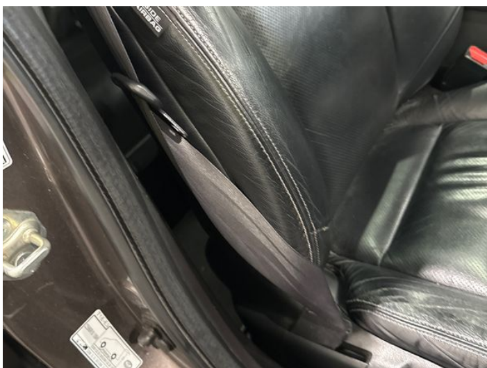
19: Seat Back Cover osf Scuffed Over 25mm
