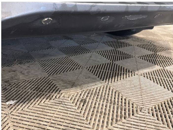
1: Bumper Front Moulding Broken Replace
