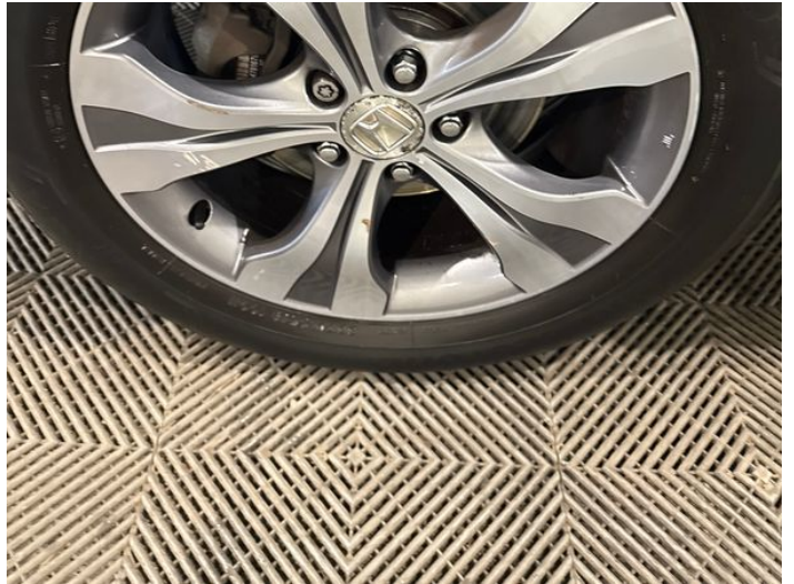
4: Wheel nsf Scratched Over 50mm
