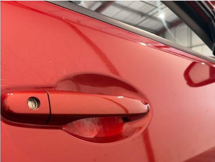
16: Door osf Scratched Over 25mm Thru Paint
