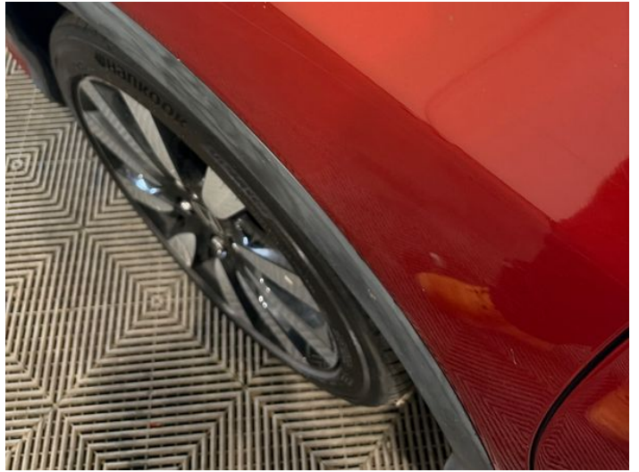
4: Wing nsf Chipped 1 To 5
