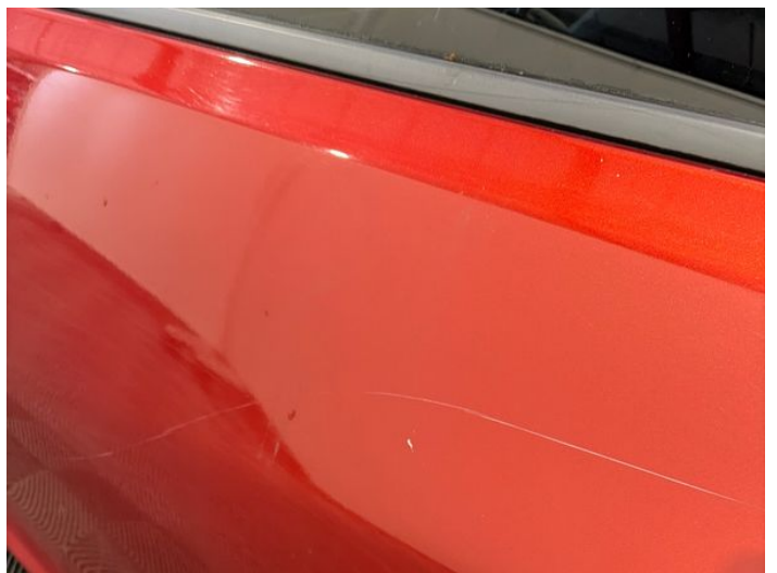
8: Door nsr Scratched Over 25mm Thru Paint
