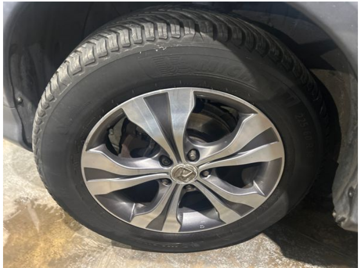
18: Wheel nsf Corroded Light
