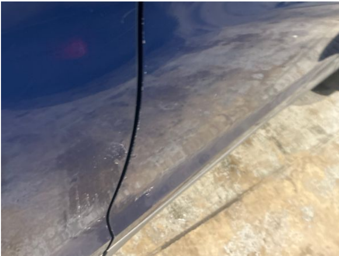
5: Door osf Chipped Edge Chip
