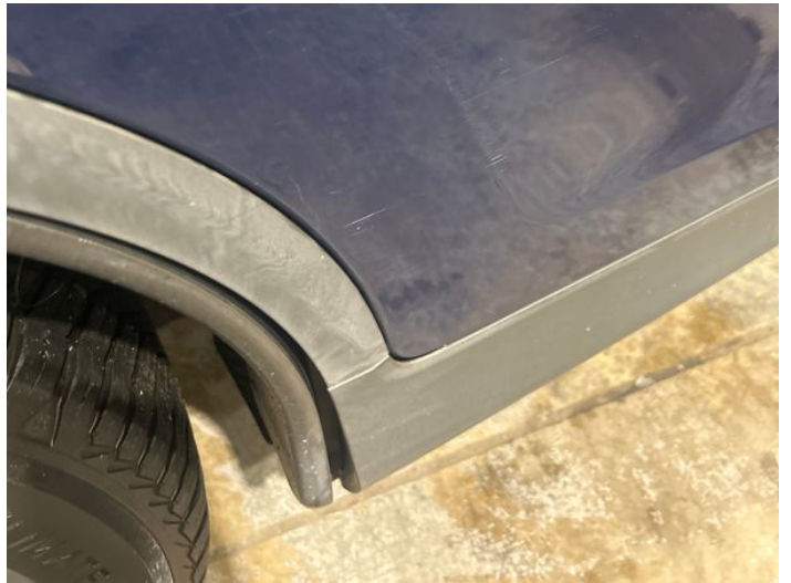
6: Door osr Scratched Over 25mm Thru Paint
