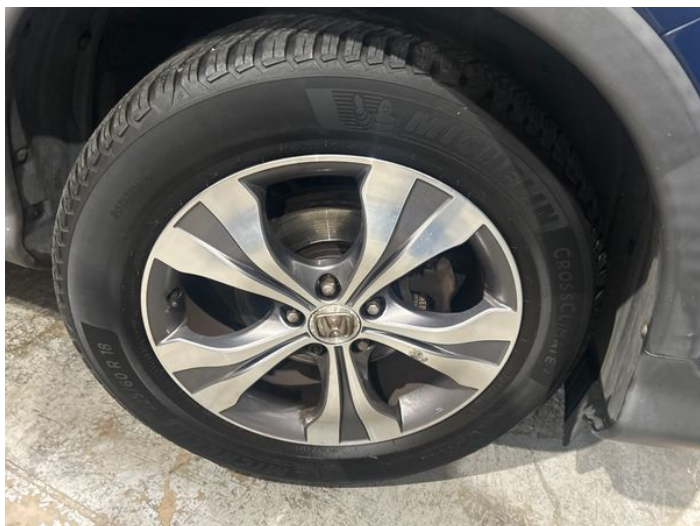
1: Wheel osf Corroded Light
