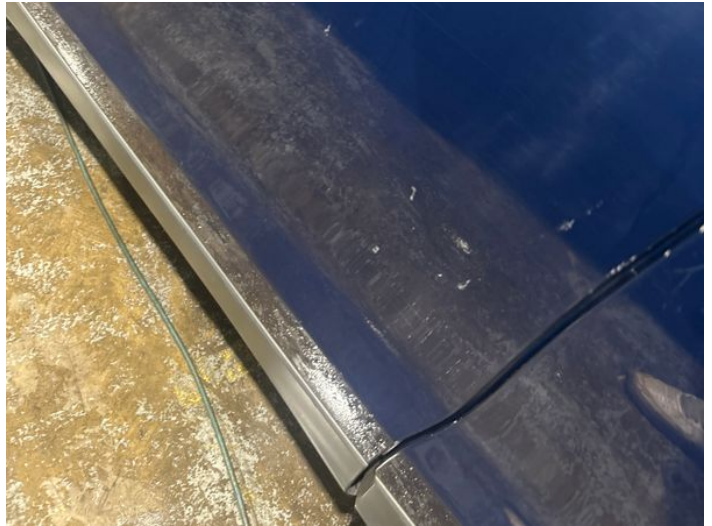
16: Door nsf Chipped Multiple Chips
