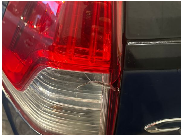
10: Lamp nsr Broken Replace
