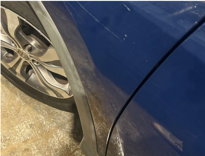
17: Wing nsf Scratched UpTo 25mm Thru Paint
