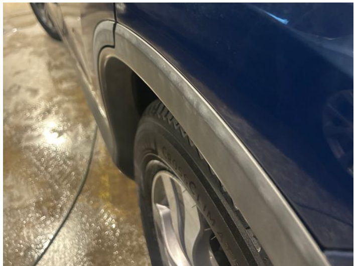
12: Qtr Panel nsr Dented Between 10mm + 30mm
