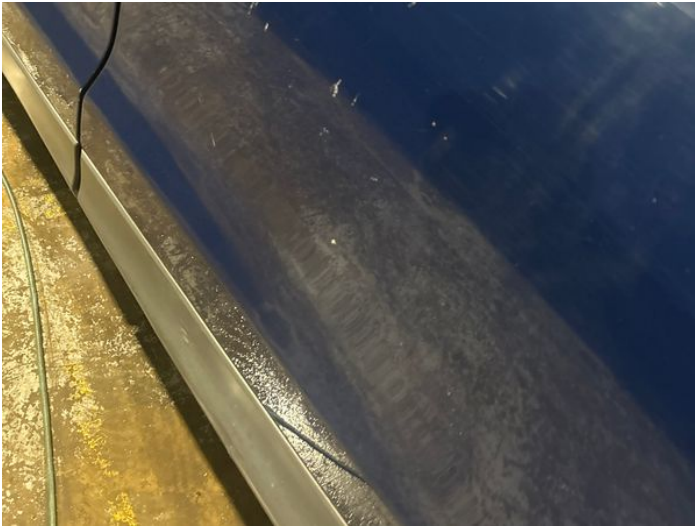
15: Door nsr Chipped Multiple Chips
