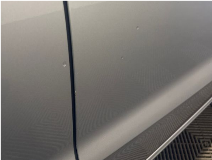
15: Door osf Chipped Edge Chip
