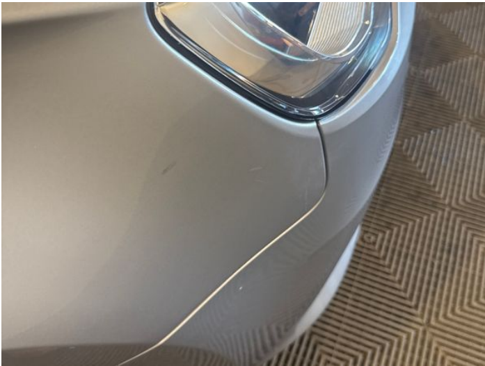
17: Wing osf Scratched Over 25mm Thru Paint
