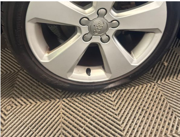
11: Wheel osr Scratched Over 50mm
